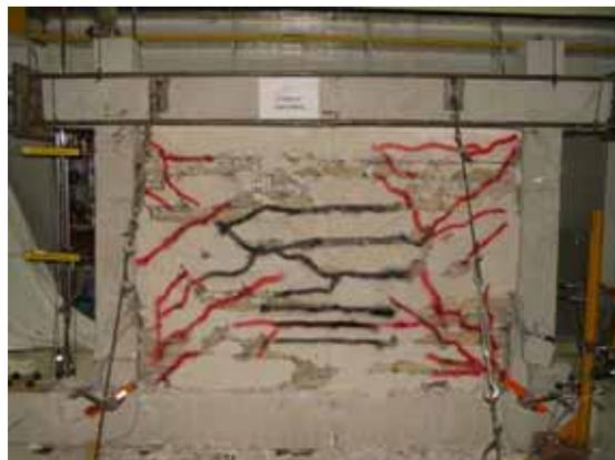
Figure 4 Failure pattern of specimen SC
