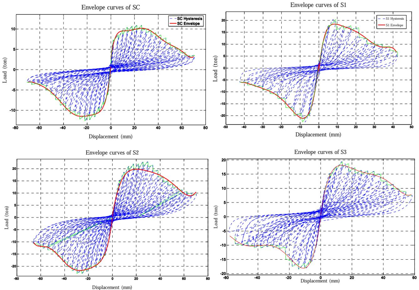
Figure 7 Hysteric Loops for Control Specimen and CFRP strengthen specimens
