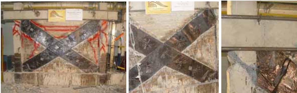
Figure 5 Crack Pattern, CFRP Delamination and Failure Mode of Specimen S2
