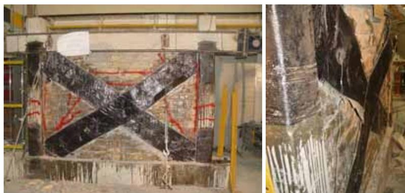
Figure 6 Crack Pattern and CFRP Delamination of Specimen S3
