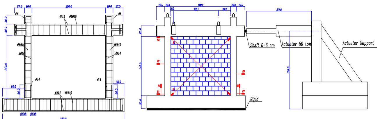
Figure1 Dimensions(Dimensions are in cm), Reinforcement Details and Specimen Test Setup
