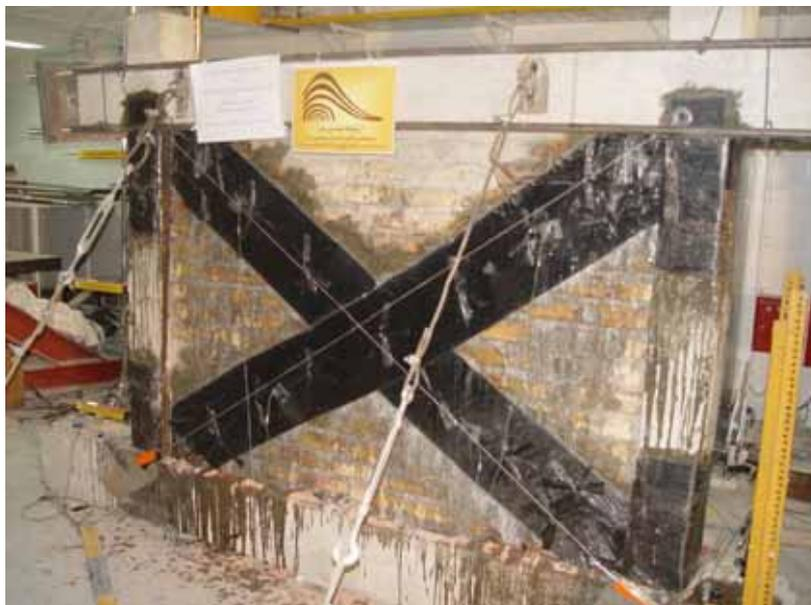
Figure 3 Retrofitting Schemes for Specimen S3
