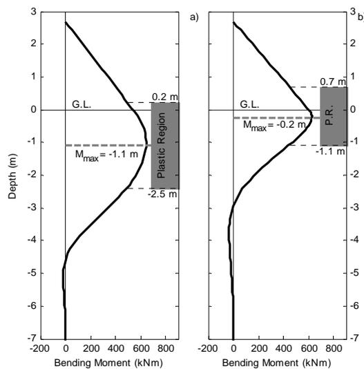
Figure 4 Bending moment profile along the length of a) SS1 at a column top lateral displacement of 19.1 cm; and b) SS2 at a column top lateral displacement of 9.4 cm
