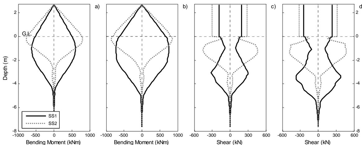
Figure 5 Envelopes of the SS1 and SS2 seismic models for a) bending moment 500 year return period; b) bending moment 2500 year return period; c) shear 500 year return period; d) shear 2500 year return period
