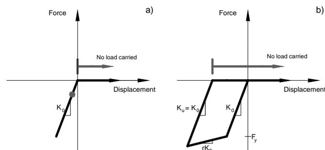
Figure 2 Compression only bi-linear soil spring hysteresis model for one side of foundation indicating displacement ranges where spring carries no force: a) prior to compressive yield; b) after compressive yield
