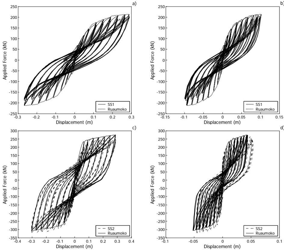
Figure 3 Cyclic force-displacement responses for a) SS1 column top; b) SS1 column base; c) SS2 column top; d) SS2 column base.
