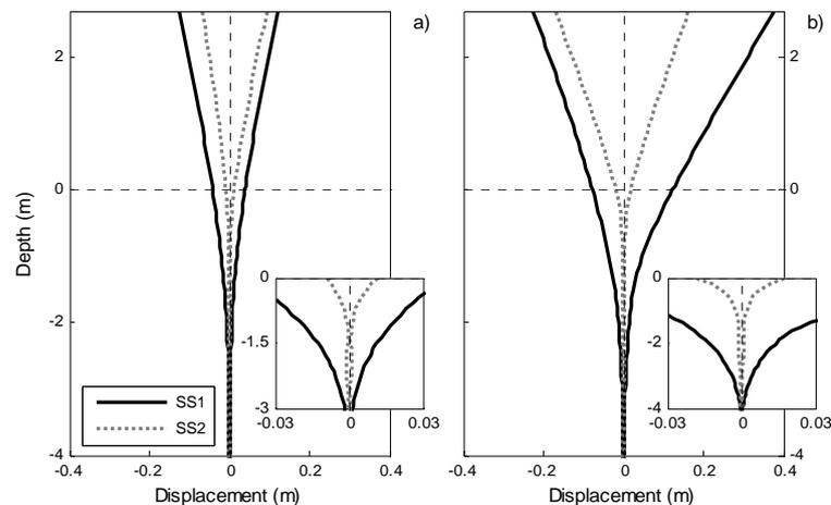
Figure 6 Horizontal displacement envelopes of SS1 and SS2 seismic models for a) 500 year return period; and b) 2500 year return period
