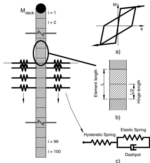
Figure 1 Seismic model layout used in Ruaumoko to represent the response of SS1 and SS2 a) column/foundation element detail; b) column/foundation moment-curvature characteristics; c) series radiation damping model
