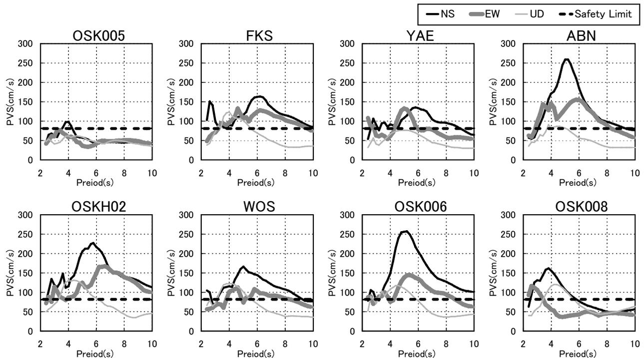
Figure 7 Pseudo velocity response spectra with 5% damping ratio and the safety limit level of the building design criterion in Japan. The safety limit level is defined for horizontal components at the engineering bedrock surface.
