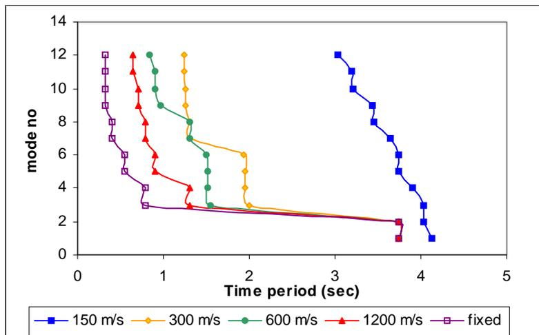
Figure 2 Comparison for modal time period for different types of soil
