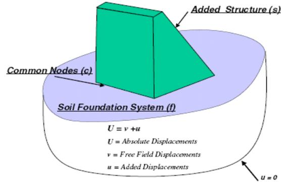
Figure 1 Soil Structure interaction model
