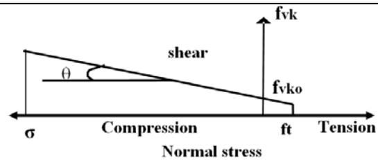
Figure 7. Mohr-Coulomb failure criterion
