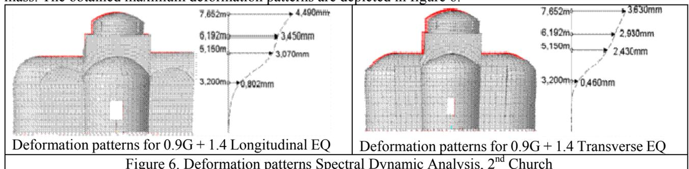
Figure 6. Deformation patterns Spectral Dynamic Analysis, 2<sup>nd</sup> Church
