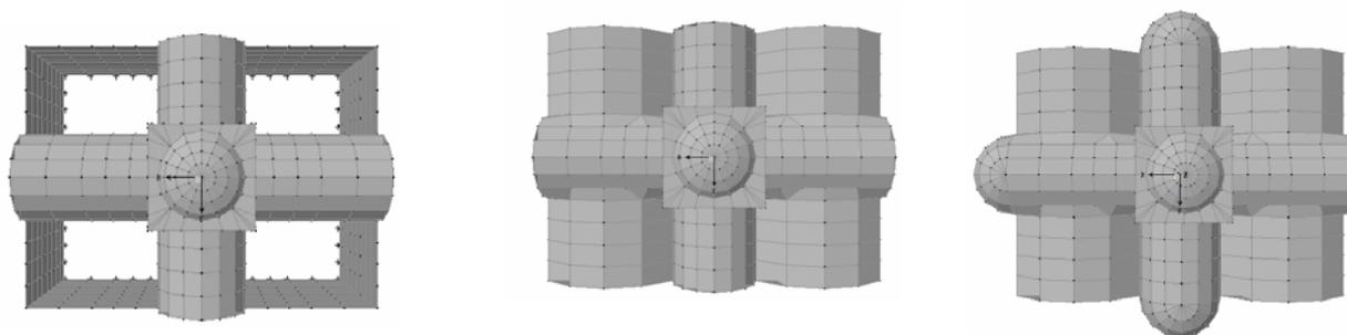
Figure 1. Plan of the Structural Formation of the superstructure of Churches of the Post Byzantine Period
