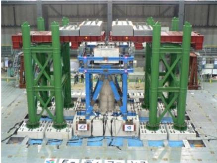
Figure 3 RC Bridge Pier Test in E-Defense
