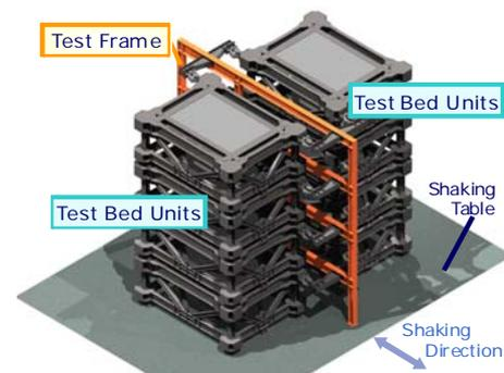
Figure 6 Multipurpose TestBed in E-Defense
