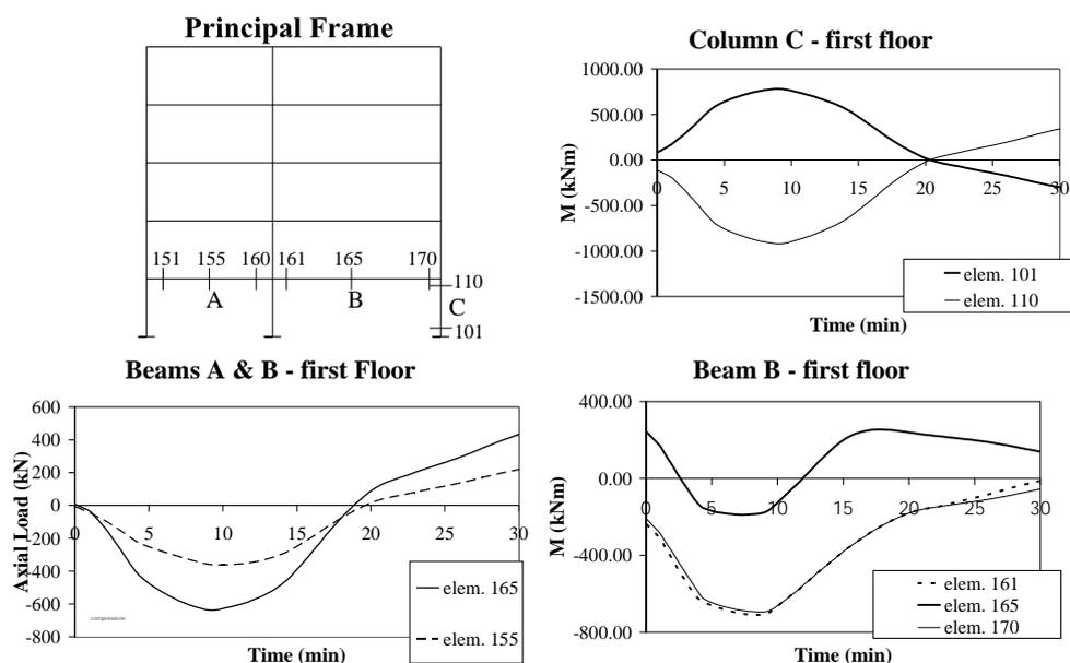
Figure 9 – Fire Case FS1: Bending moment and Axial load in beams and columns at the first storey
