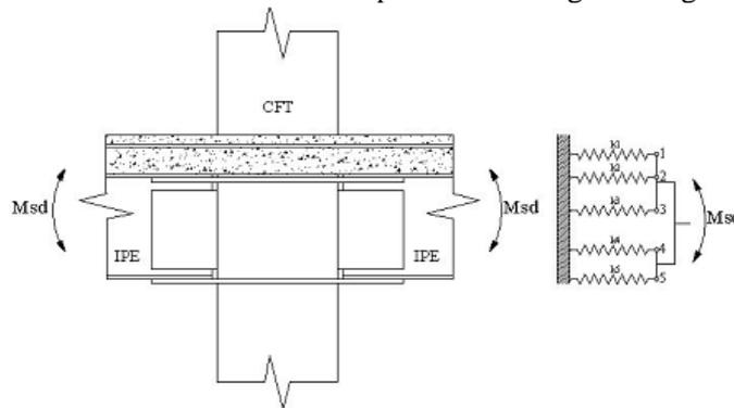
Figure 4 Mechanical model of a steel-concrete composite interior joint including sagging moments
