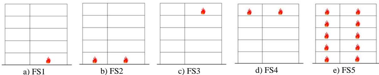
Figure 8 Fire scenarios considered in thermal analyses
