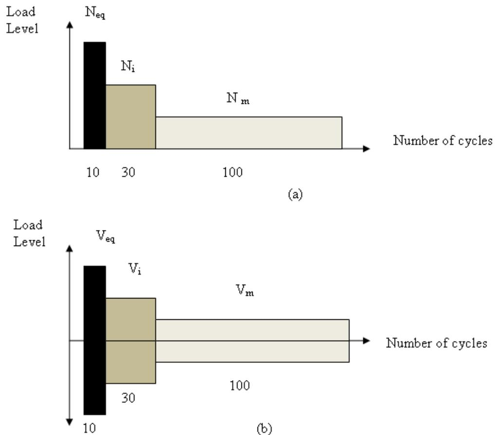
Figure 3 Cyclic loading profile for (a) Tension or combined tension and shear tests, (b) Direct shear tests
