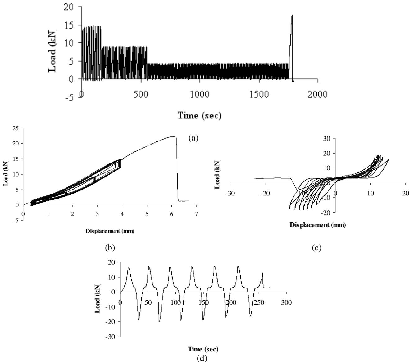
Figure 5 (a) Typical loading profile for 50% cyclic tension test, (b) Load-displacement curves for undercut expansion anchor subjected to 50% cyclic tension, (c) Load-displacement curves for screw type anchor subjected to 75% cyclic shear, and (d) Typical loading profiles for 75% cyclic shear test.
