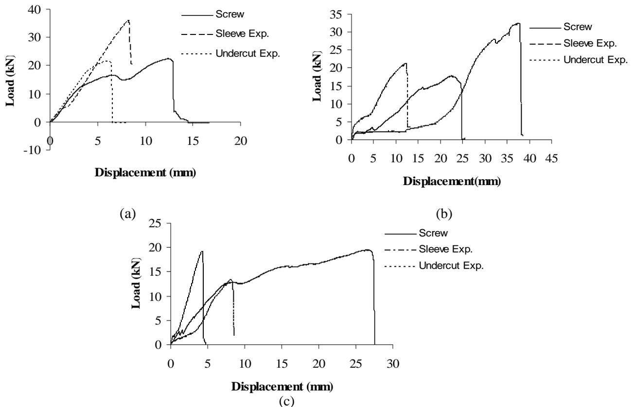
Figure 4 Static test results (a) Typical anchor tensile force-axial displacement, (b) Anchor shear force-lateral displacement, and (c) Anchor resultant force-resultant displacement under combined load
