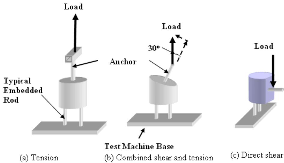
Figure 2 Typical test set-up and applied loadings
