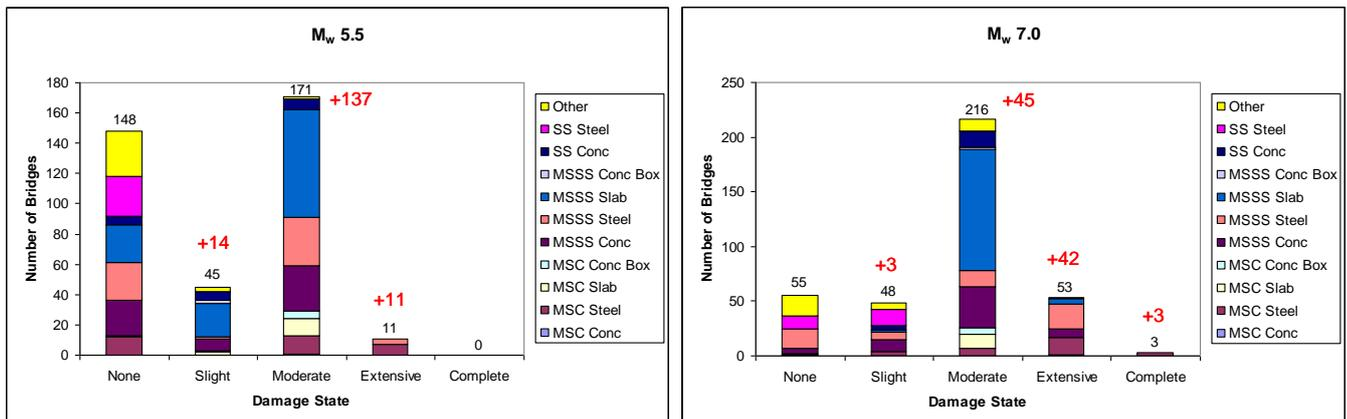
Figure 5 Damage state distribution by bridge type and damage state for  $M_w$  5.5 and 7.0 events.
