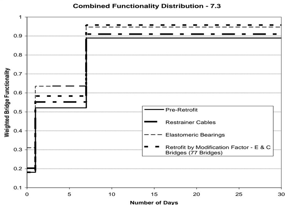
Figure 7 System functionality at 0, 1, 7, and 30 days for pre-retrofit and various retrofit measures for M<sub>w</sub> 7.3 event.
