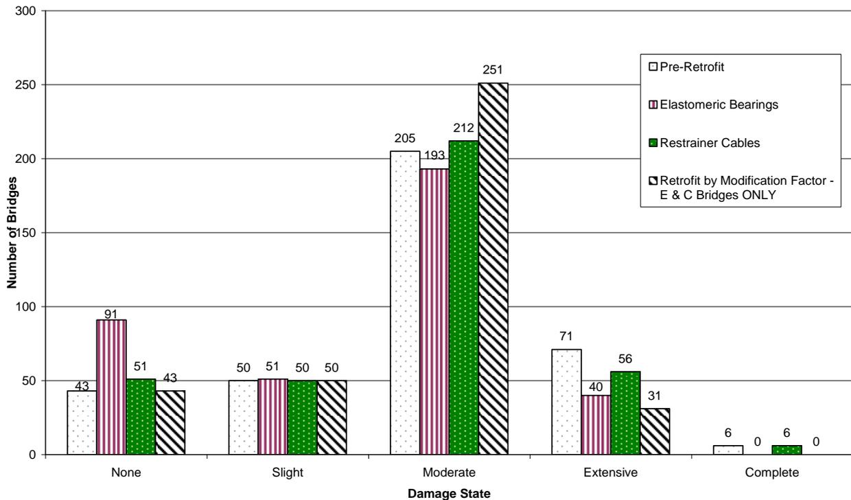
Figure 6 Distribution of bridges by damage state and retrofit approach for a Mw 7.3 event.
