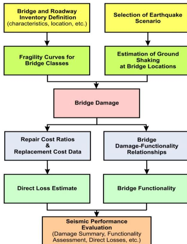
Figure 1 Schematic of general seismic risk assessment methodology applied
