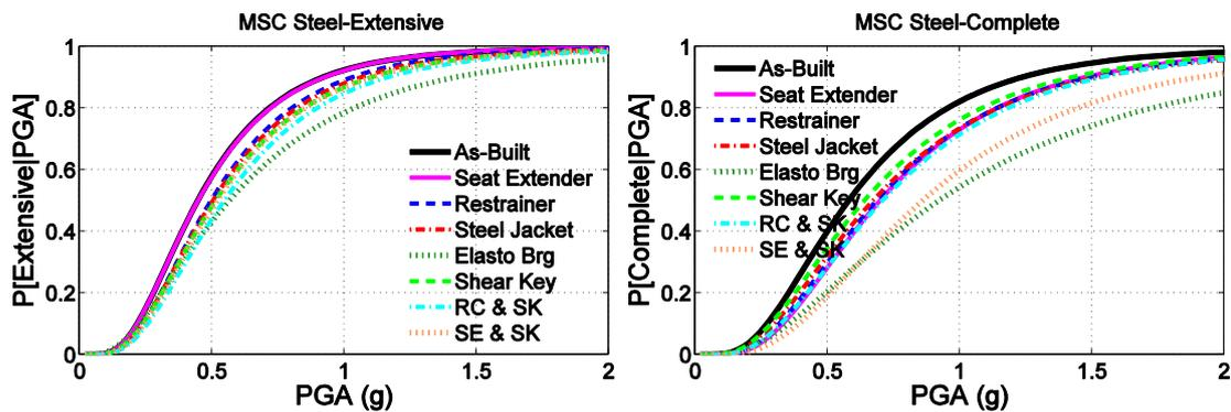
Figure 3 Comparison of the fragility of the MSC steel bridge with various retrofit measures at two damage states
