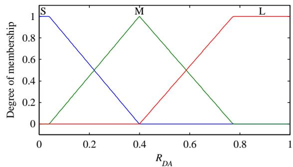
Figure 7 Membership functions for  $R_{DA}$
