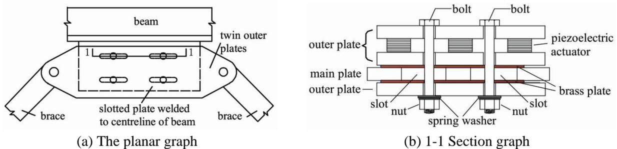
Figure 1 Piezoelectric friction damper
