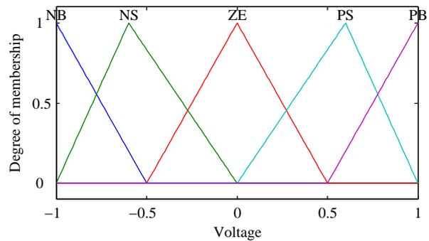
Figure 3 Membership functions for voltage
