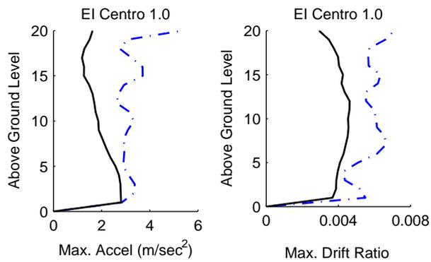
Figure 8 Responses under EI Centro earthquake
