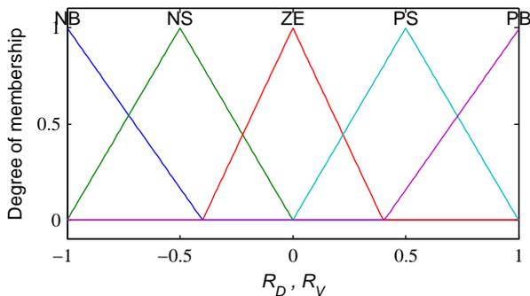
Figure 2 Membership functions for  $R_D, R_V$
