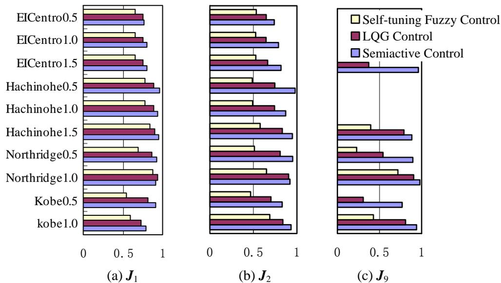
Figure 12 Bar chart comparing the evaluation criteria for various controller
