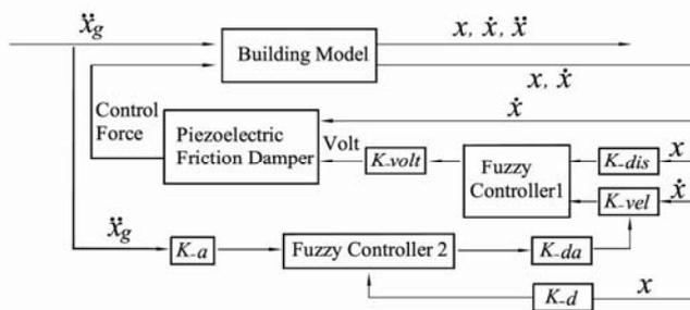
Figure 4 Diagram of self-tuning fuzzy control system
