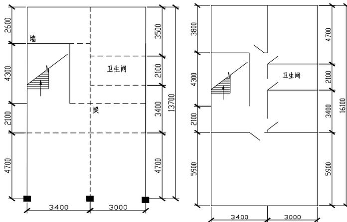
a) Planar graph of the first floor b) The planar graph of the second floor
