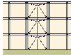
Fig.42 Adding damper for reinforcement
