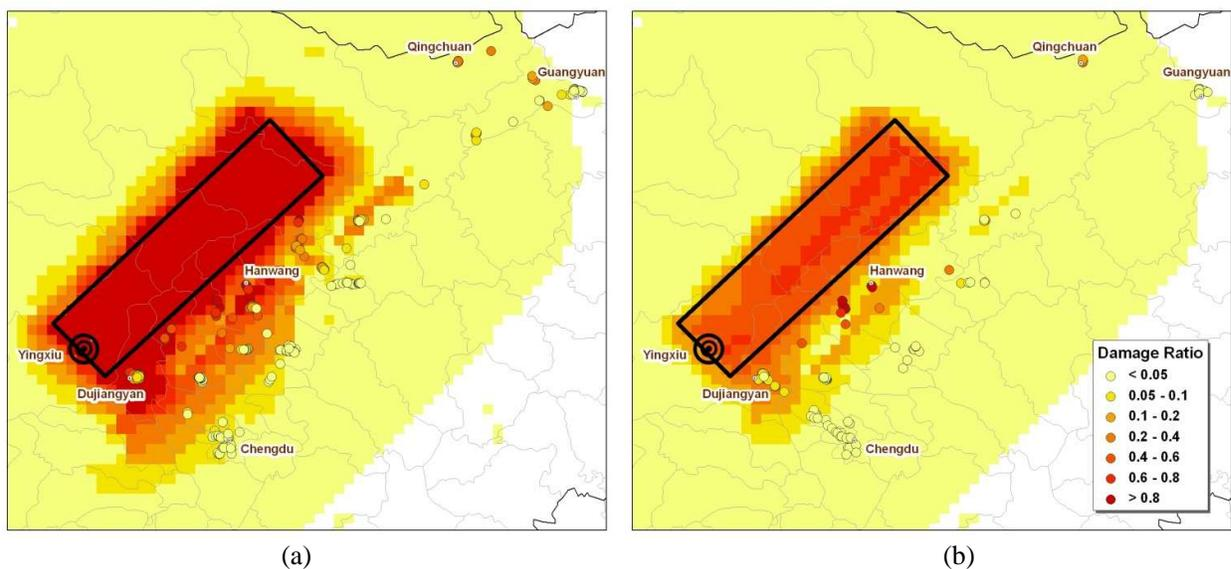
Figure 3: Comparison of the observed (colored circles) and simulated damage (background color) for (a) mid-rise CM buildings and (b) mid-rise RC buildings
