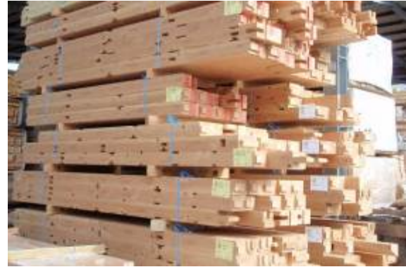
Fig. 5 Pre-cut notched joints
