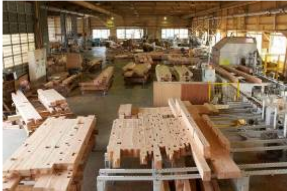
Fig. 5 Pre-cut notched joints
