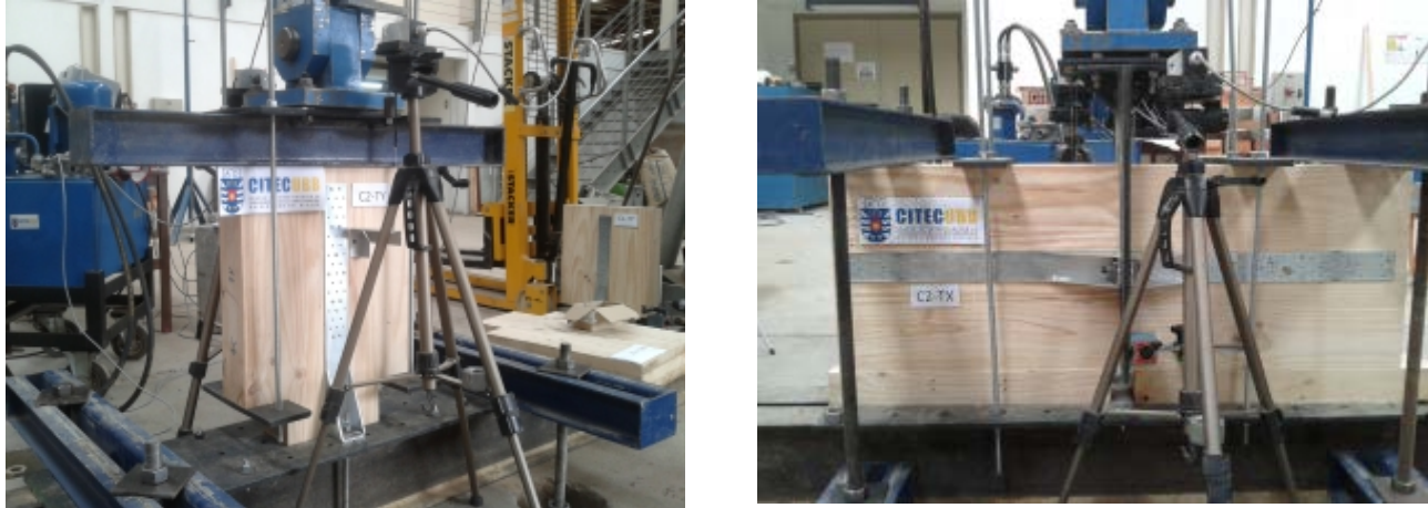
Figure 1: Parallel to grain hold down cyclic test setup (left) and perpendicular to grain hold down cyclic test setup (right)
