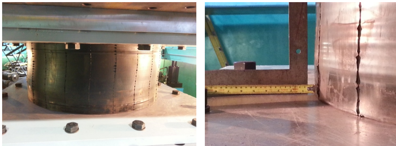
Fig. 6 – Distortion of LRB after 2D-400% strain test
