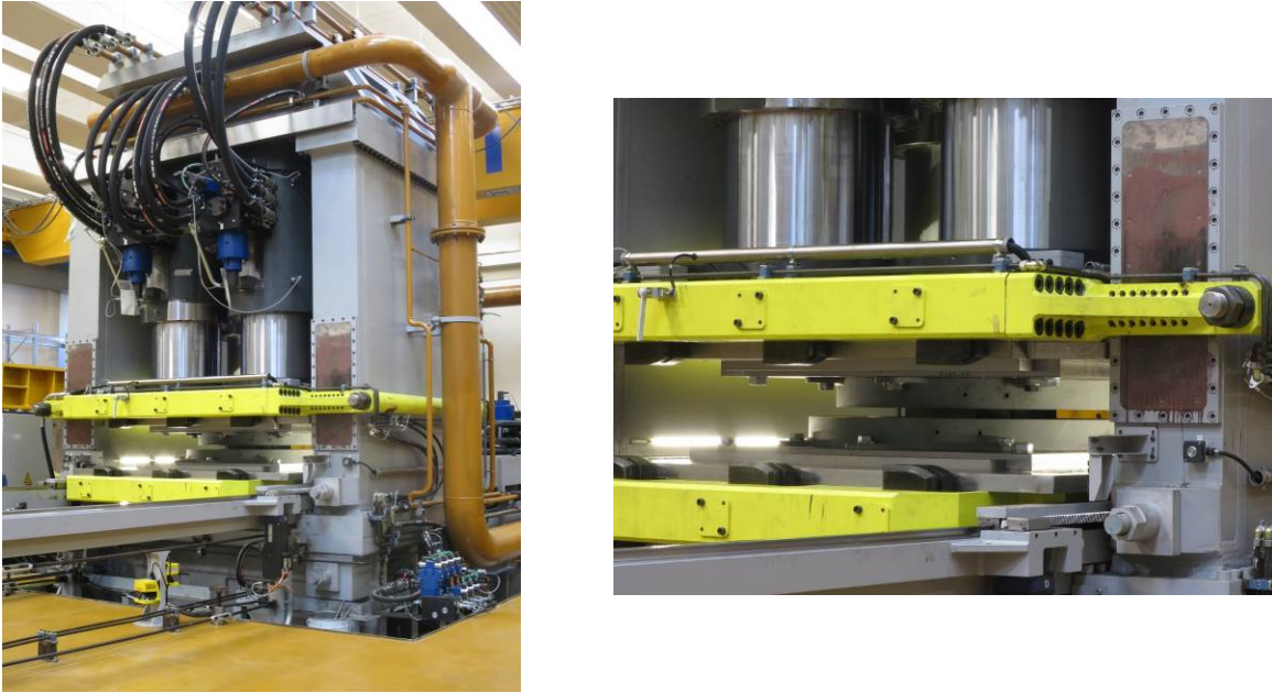
Fig. 9 - Biaxial test system - FIP Industriale Dynamic Test Laboratory.
