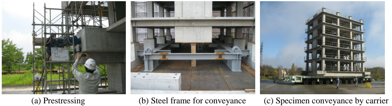
Fig. 6: Specimen conveyance procedure
