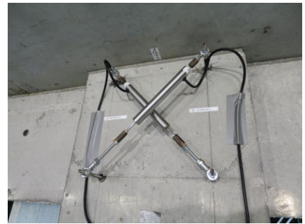
(f) Beam-column joint deformation
