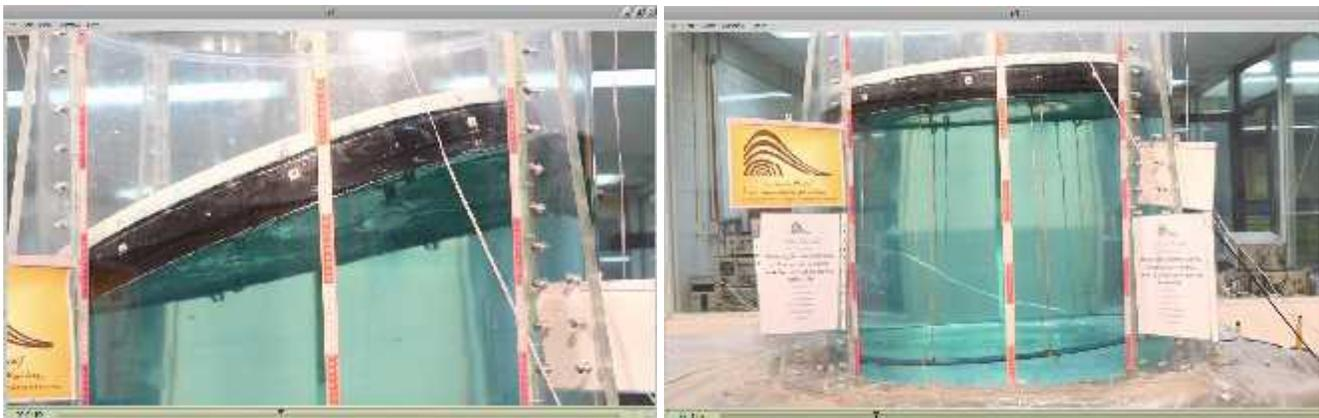
Fig. 6- The side view of the tank from the position of camera 1 for  $H_L=70$  cm, at the instant of maximum sloshing height due to harmonic excitation with amplitude of 4 mm and frequency of 0.95 Hz in both non-baffled (NB) (left) and baffled (right) cases with baffle width of 7 cm (BW7)
