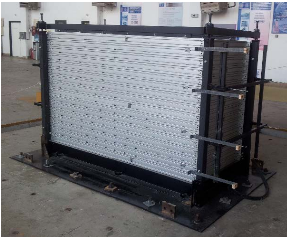
Figure 1. The laminar box designed and constructed in IZIIS
