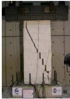
Fig. 8 – Specimen CS 05 at the end of the test (left) and comparison among the base shear vs. top displacement curves obtained from experimental test and numerical simulation with the current (centre) and the new (right) TREMURI constitutive model for wall CS 05
