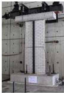
Fig. 10 – Wall EC_COMP_2: view of the specimen (left) and comparison among the base shear vs. top displacement curves obtained from experimental tests and numerical simulation with the current (centre) and the new (right) TREMURI constitutive model
