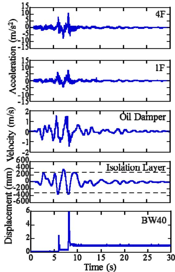
Fig. 5 Response of Superstructure, Isolation Devices and Retaining Walls under Takatori 65% Excitation with Pounding to BW40 with Rubber Blocks (Case 2)
