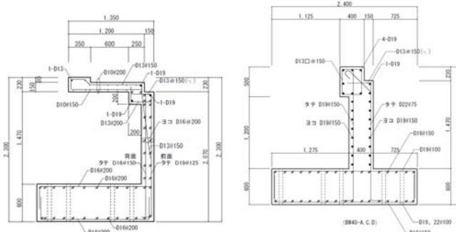
(b) Retaining Wall BW20 (c) Retaining Wall BW40
