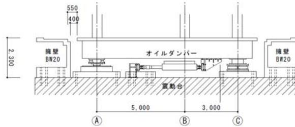
(a) Sectional View (Section 3, Isolation Layer with Retaining Walls)
