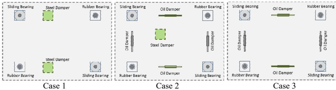
Fig. 3 Setup of Isolation Devices
