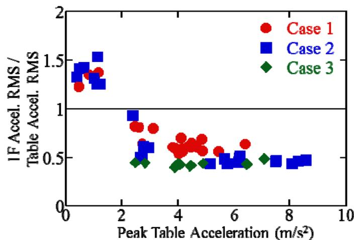
Fig. 6 Decrement of Floor Acceleration by Base-Isolation
