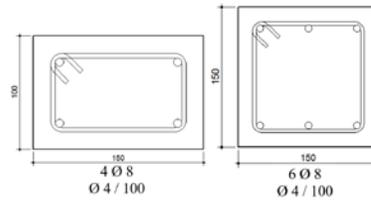
Fig. 4 - Reinforcement details of the column and beam cross sections
