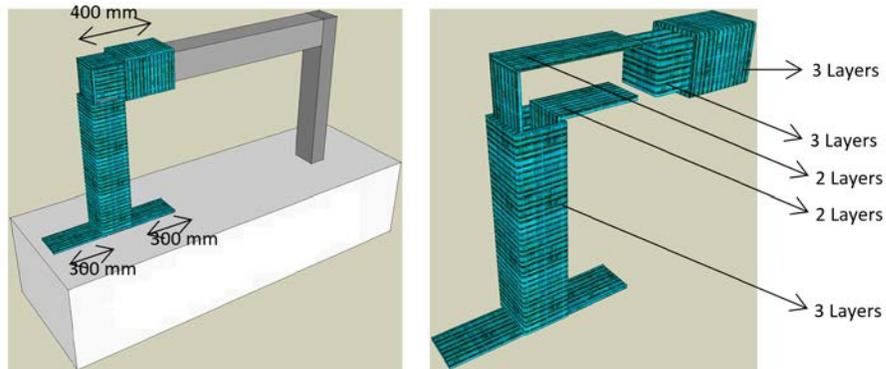
Fig. 3 - Schematic representation of CFRP sheets
