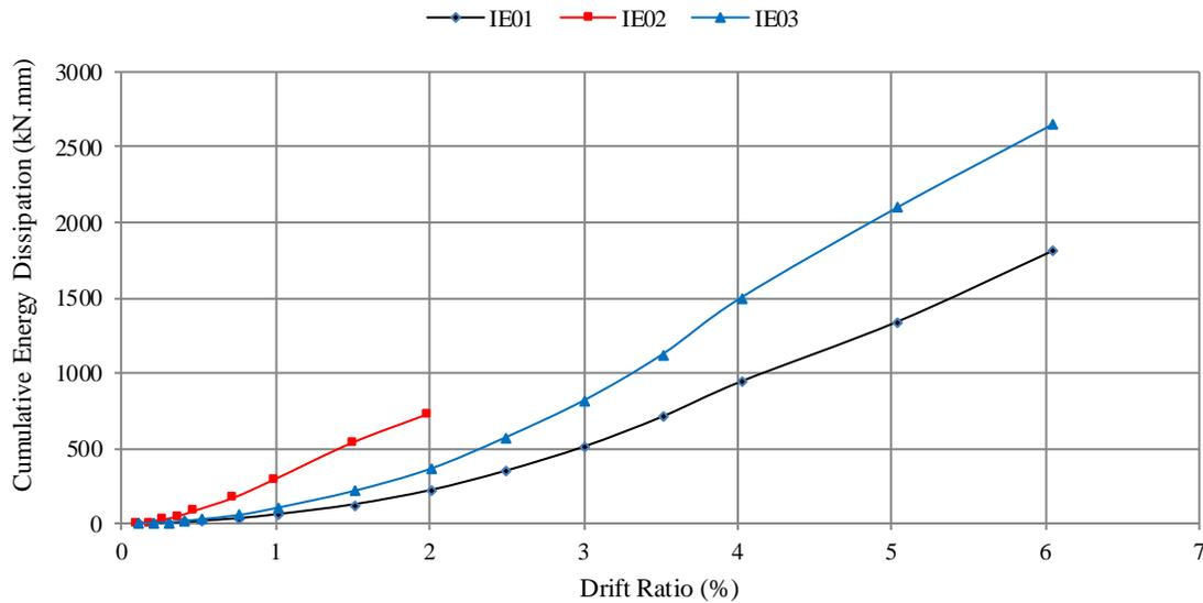
Fig. 12 - Cumulative energy dissipation capacity of the tested specimens
