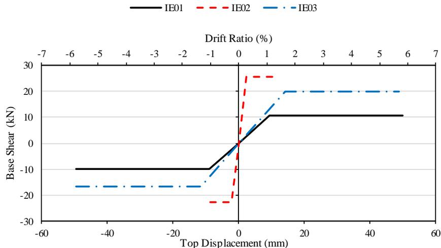
Fig. 11 - Idealized bi-linear representation of the envelope curves
