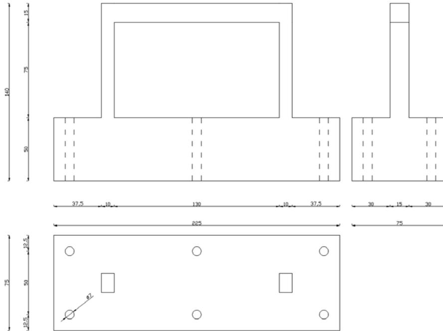
Fig. 5 – Geometric properties of the beam, columns and foundation of the test specimens
