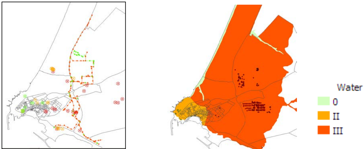
Fig. 6 – Impact of the earthquake in the water supply system: left) direct damage to reservoirs and piping; right) disruption to the whole system.
