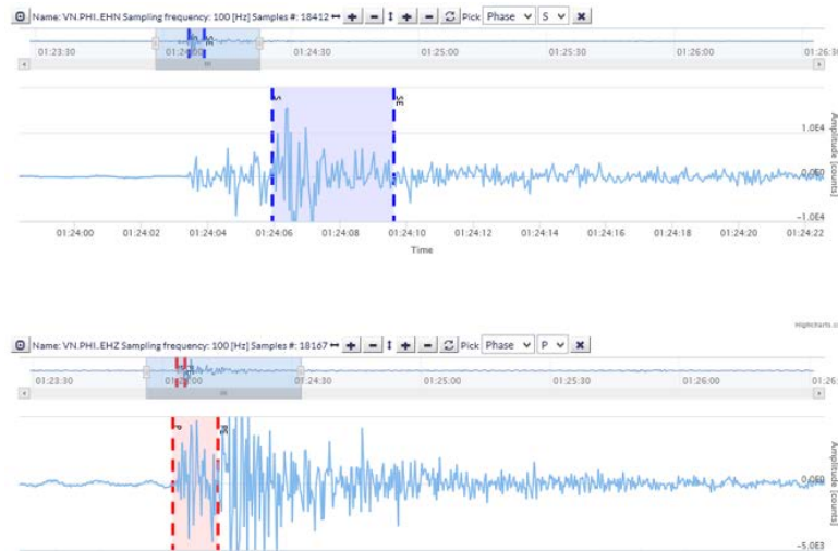
Fig. 5 – Picking tool demonstration, P-wave phase (bottom) and S-wave phase (top)
