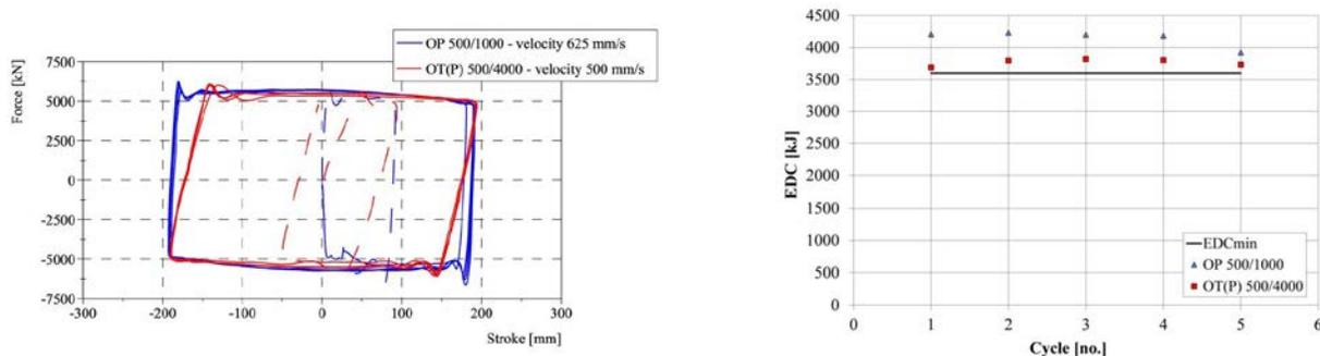
Fig. 13 - Damping efficiency test. Hysteretic loops for OT(P) 500/4000 (left) and EDC compared with the minimum allowable  $EDC_{min}$  (right) for both dampers.
