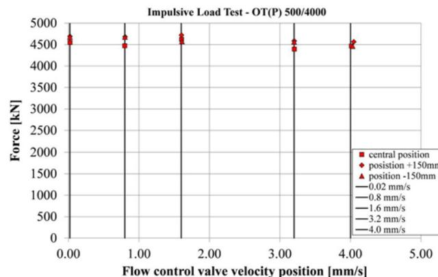
Fig. 9 – Impulsive load test results of OT(P) - Force vs. flow control valve velocity
