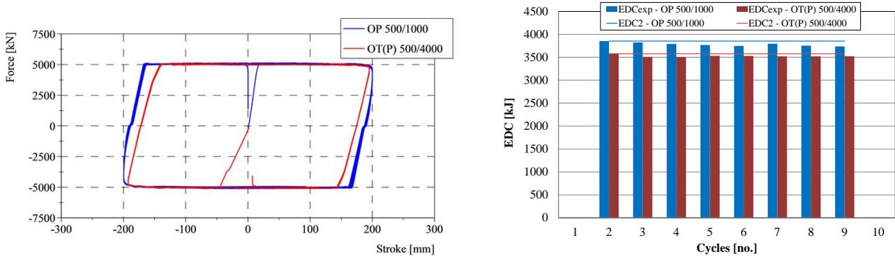
Fig. 10 - Dynamic loading test results: Hysteretic loops (left) and energy dissipation results compared with the 2<sup>nd</sup> loop cycle (reference cycle).
