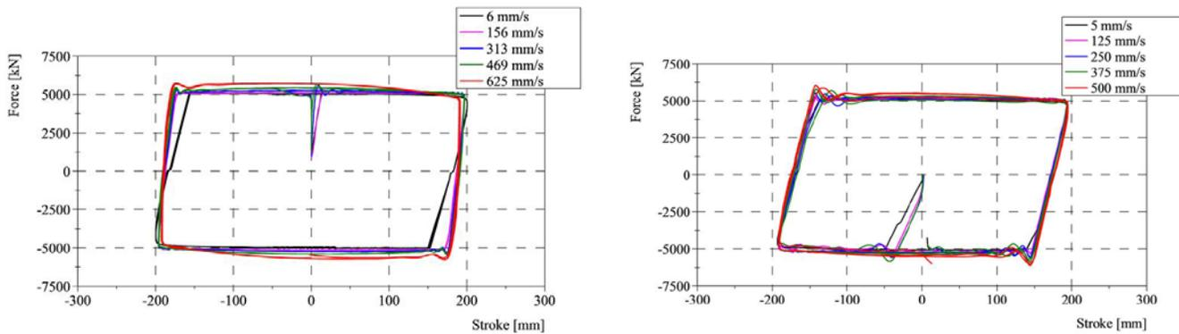
Fig. 12 – Constitutive Law test - Force vs. displacement curves at all velocities, for OP 500/1000 (left) and OT(P) 500/4000 (right)
