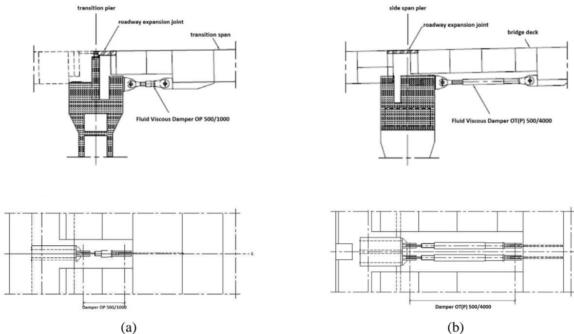
Fig. 3 – Positioning of the two types of FVDs in the transition pier (a) and side span pier (b) [8].
