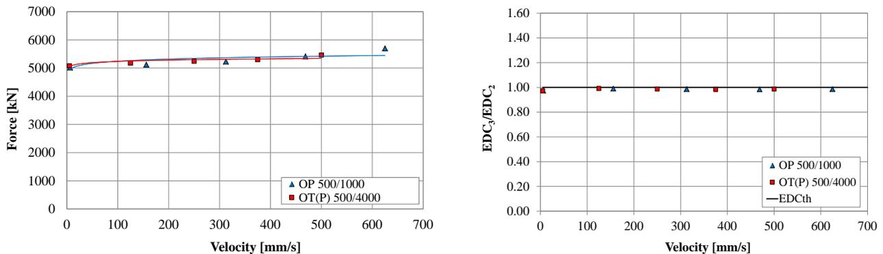
Fig. 11 - Constitutive law test results for both dampers in ambient temperature. Force vs. velocity curve (left) and normalized energy dissipation values (right).
