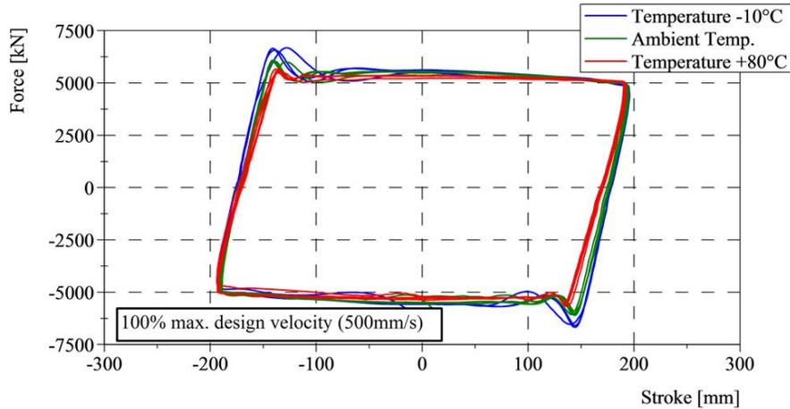
Fig. 16 – Comparison of Damping Efficiency Test results at  $-10^{\circ}\text{C}$ , ambient temperature and  $+80^{\circ}\text{C}$ . Hysteresis loops for damper OT(P) 500/4000.
