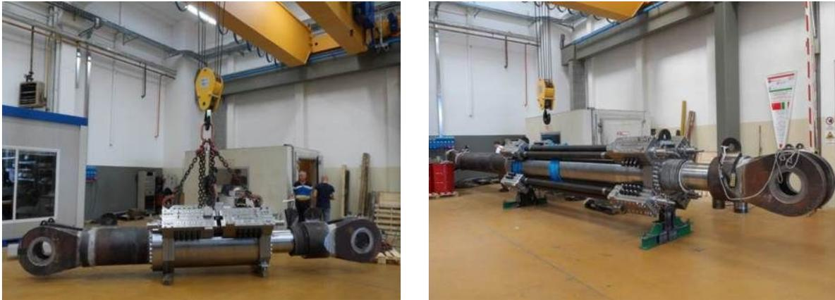
Fig. 6 – FVDs arrived at FIP Industriale Laboratory to be tested. Damper type OP 500/1000 (left) and damper type OT(P) 500/4000 (right)
