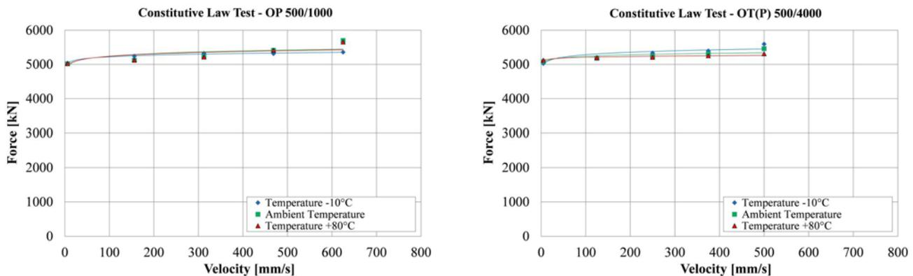
Fig. 15 - Comparison of Constitutive Law Test results at  $-10^\circ\text{C}$ , ambient temperature and  $+80^\circ\text{C}$ . Force vs. velocity curves for damper OP 500/1000 (left) and damper OT(P) 500/4000 (right).
