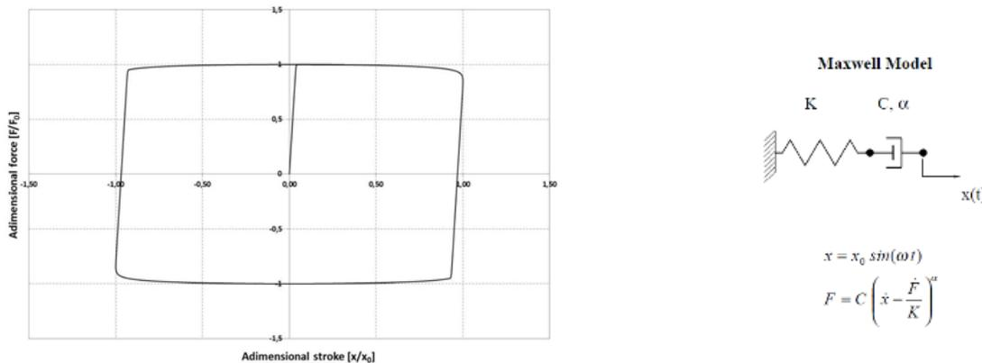
Fig. 4 – Typical hysteresis loop for viscous damper (left), Damper constitutive law and mathematical model (right).
