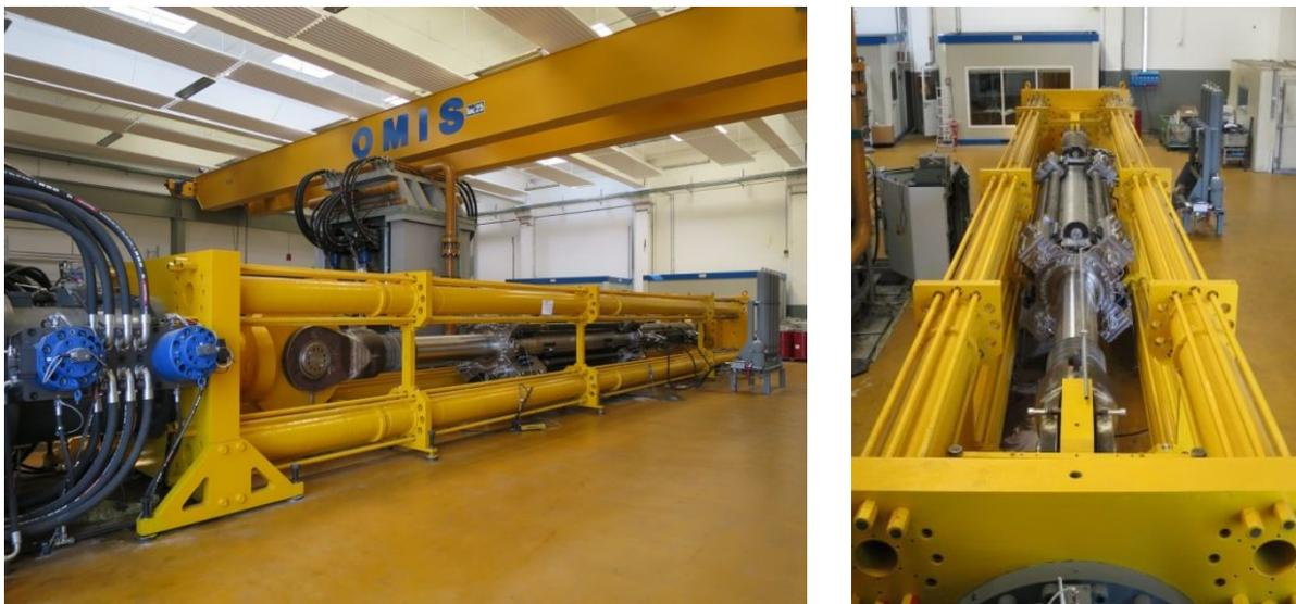
Fig. 7 - Viscous damper OT(P) 500/4000 under testing at FIP Industriale Laboratory.
