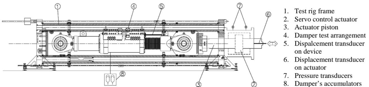
Fig. 8 – Test set-up scheme
