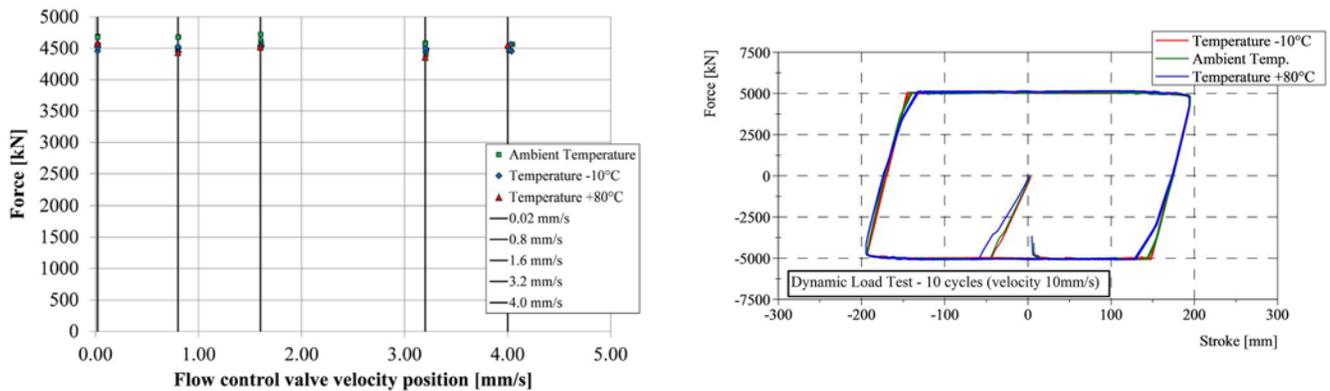
Fig. 14 – Comparison of different temperatures for damper type OT(P) 500/4000 - Impulsive Load Test (left) and Dynamic Loading Test (right).
