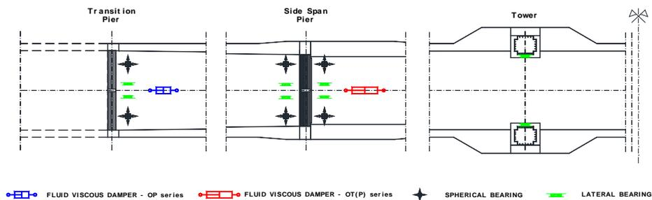
Fig. 2 - Bridge viscous dampers and bearings layout (one half of the bridge is represented, the layout is almost symmetrical, apart the number of viscous dampers on the transition piers).
