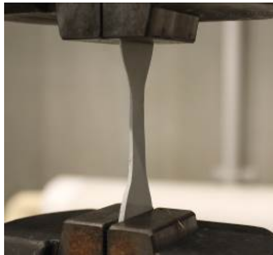
Fig. 3 – Axial tensile tests of paint
