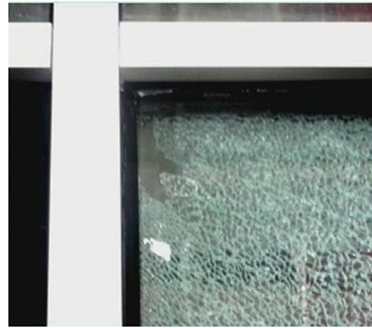
(a) (b) Fig. 3 – (a) Load-drift relationship and (b) failure mode on façade B
