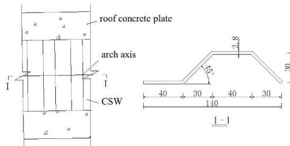
(b) Dimensions of corrugated steel web (unit: mm)
