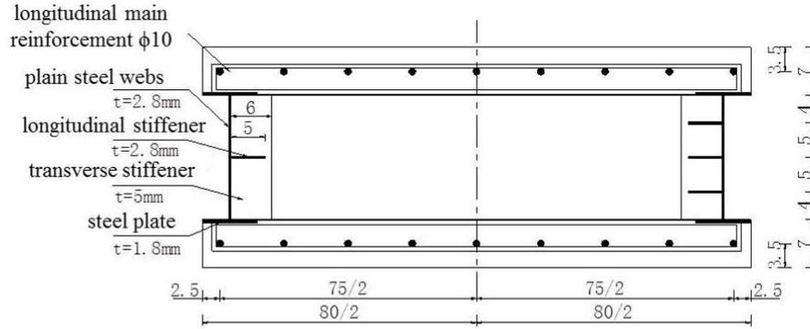
(a) Cross section of RC-PSW arch model (unit: cm)
