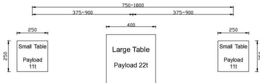
(b) Arrangement plane view of shaking table system (unit: cm)
