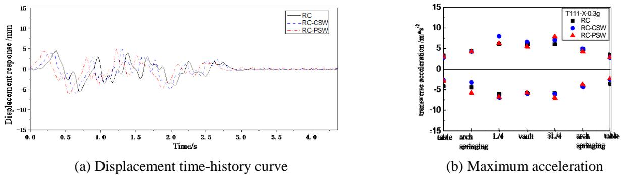
Fig. 9 – Comparison of seismic response among three models under longitudinal seismic excitation (PGA=0.3g)
