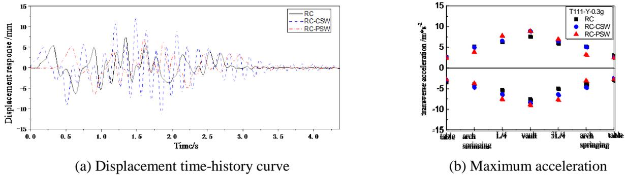
Fig. 8 – Comparison of seismic response among three models under transverse seismic excitation (PGA=0.3g)
