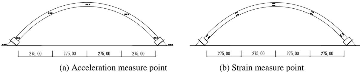
Fig. 7 – Measure point arrangement (unit: cm)
