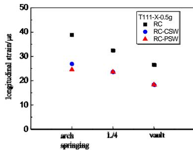
Fig. 10 – Comparison of concrete strain under longitudinal seismic excitation (PGA=0.5g)
