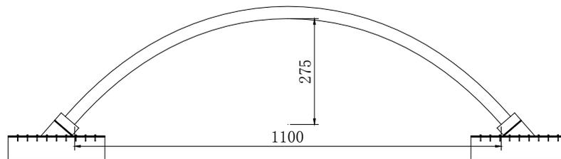
Fig. 2 – Schematic illustration of elevation arrangement for RC arch model (unit: cm)
