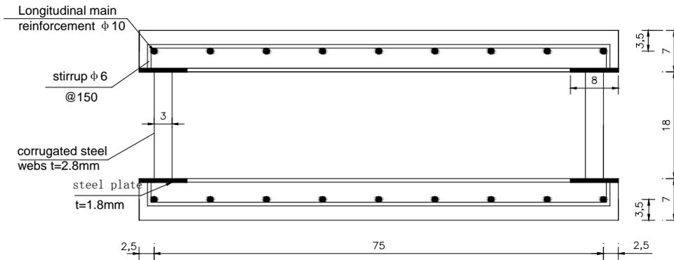
(a) Cross section of RC-CSW arch model (unit: cm)
