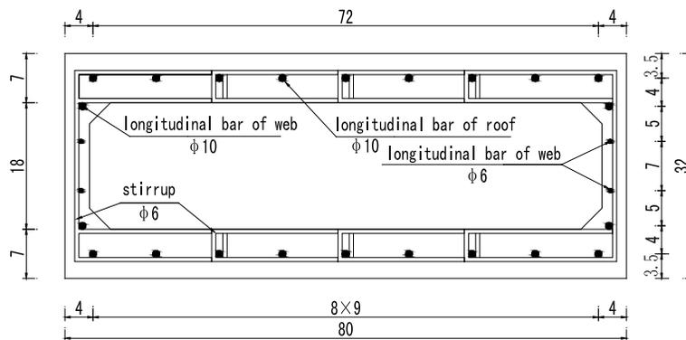
(a) Cross section of RC arch model (unit: cm)
