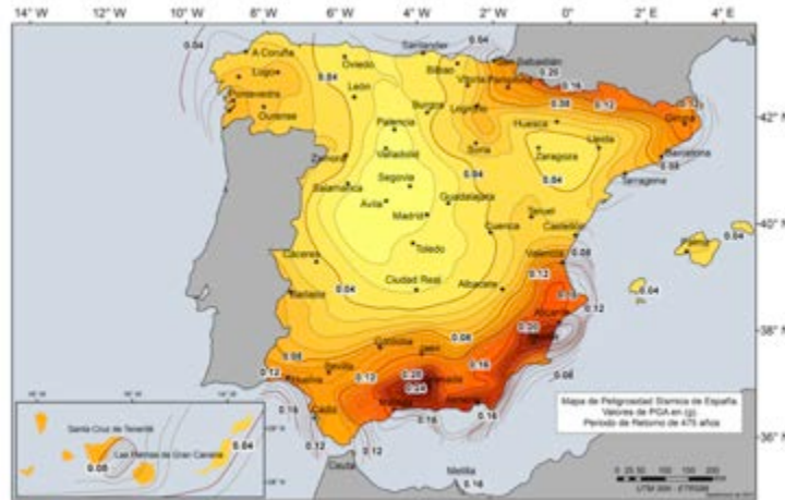
Figure 6. Hazard map derived in the study in terms of PGA (g) mean of the logic tree and Montecarlo simulation for a return period of 475 yrs .
