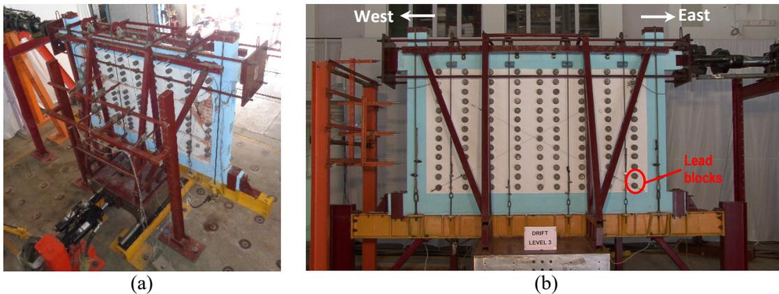
Fig. 3 – Typical test setup for wall specimens: (a) out-of-plane loading, and (b) in-plane loading
