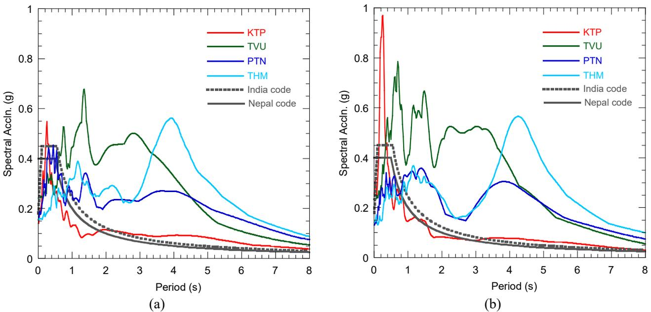
Fig. 4 – Comparison of 5% damped acceleration response spectra of recorded ground motions of main shock at KTP (rock site), TVU (soil site), PTN (soil site) and THM (soil site) with the Indian and Nepalese seismic code specified elastic design response spectrum for the design basis earthquake in soft soil site: (a) N-S component, and (b) E-W component
