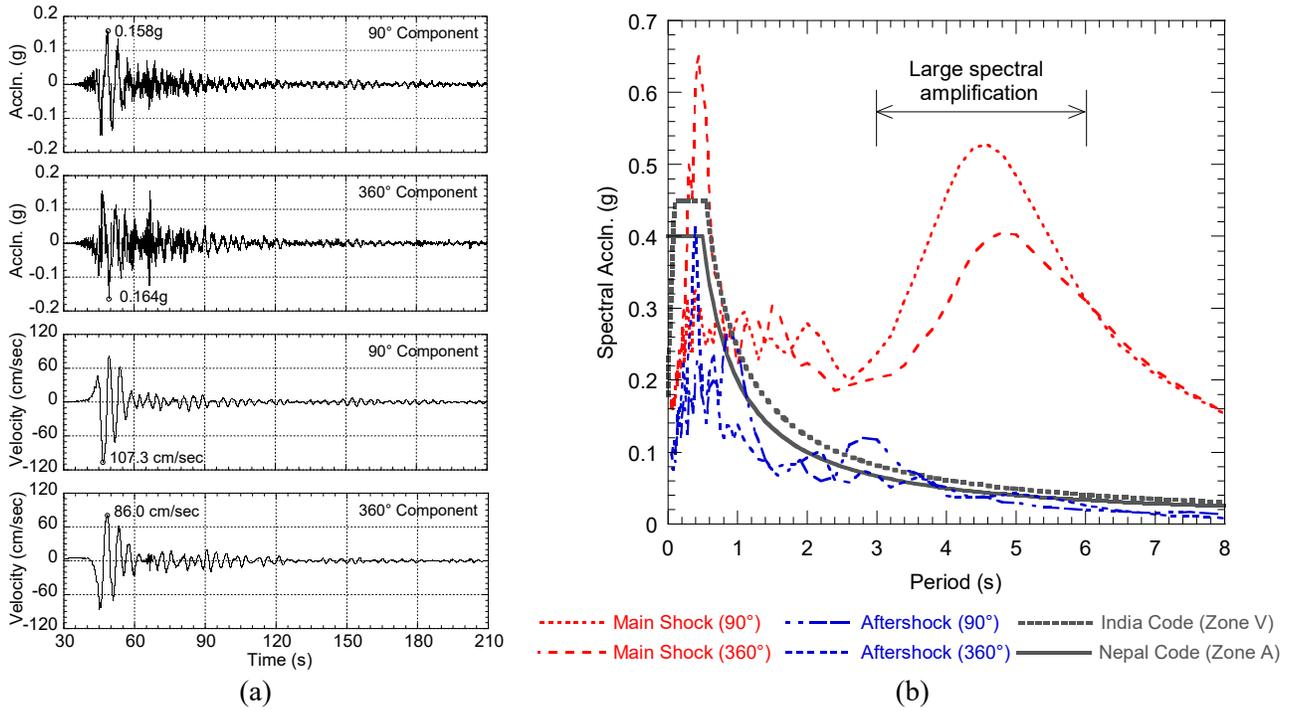
Fig. 3 – (a) Acceleration time histories for the main shock of the 25 April 2015 event recorded at Kathmandu, and (b) Comparison of 5% damped acceleration response spectra of recorded ground motions of main shock and M7.3 aftershock with the Indian and Nepalese seismic code specified elastic design response spectrum for the design basis earthquake in soft soil site
