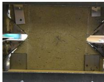
Pic. 5 - Crack at 0.2mm of displacement
