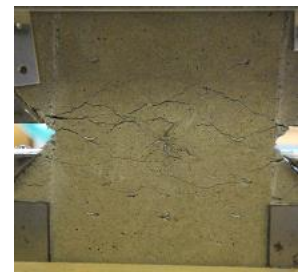
Pic 6 - Crack at 1.5mm of displacement
