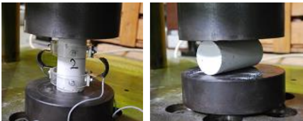
Pic. 1 - Material testing of mortar
