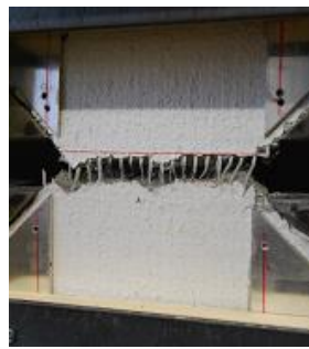
Pic. 8 - Ultimate state on tension test of mortar element specimen
