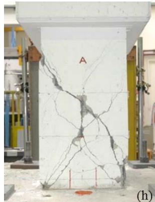
Fig. 4 – Lateral load versus drift cyclic response and final damage state, P1 (a,b), P2 (c,d), P3 (e,f), P2 (g,h)
