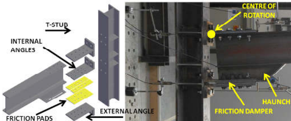
Fig. 1 –Typical layout of a FREEDAM connection
