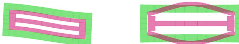
3 rd modal shape T=0.119 sec F= 8.38 Hz 5 th modal shape T=0.091 sec F= 10.98 Hz
