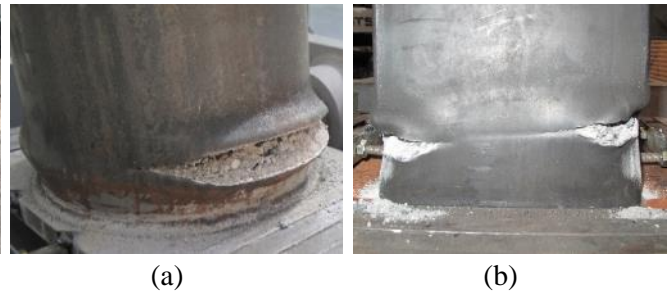
Fig. 5 – Fracture of the circular(a)/rectangular(b) CFST during a cyclic test
