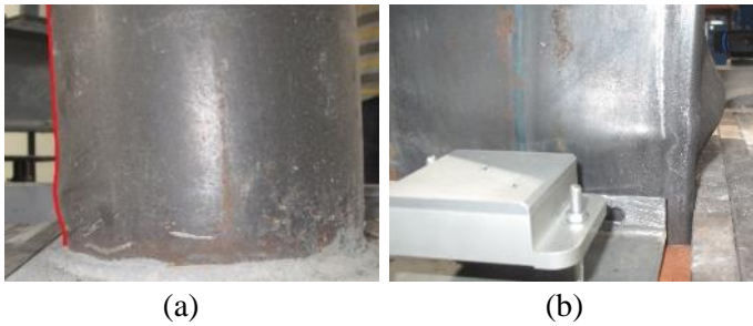
Fig. 4 – Local buckling of the circular(a)/rectangular(b) CFST in a monotonic test
