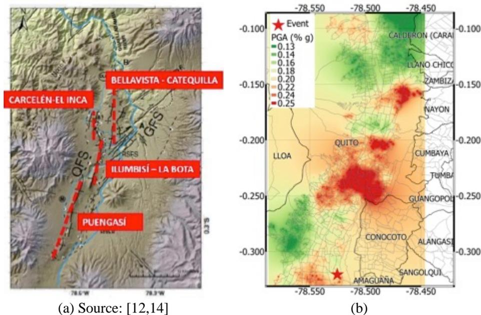
Fig. 1 – (a) Segments of the Quito Fault System; (b) Example of one realization of the ground motion field for the rupture selected for the analysis
