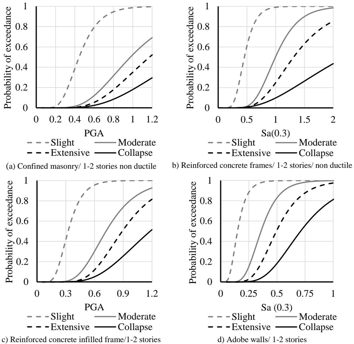
Fig. 3 – Example of fragility functions used for the analysis
