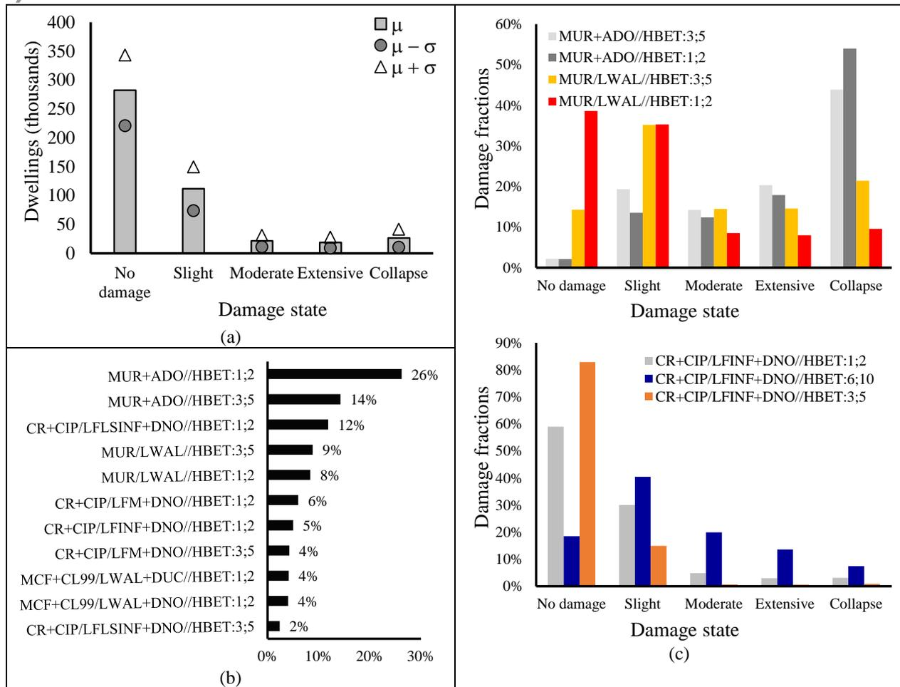
Fig. 5 – (a) Total distribution of damages; (b) contribution of building typologies to the total number of collapsed buildings; (c) damage fractions for various building types
