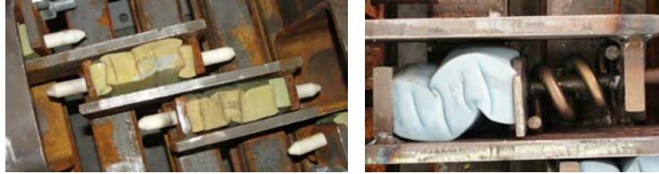
Figure 1 (Left) Standard equidistant configuration, (Right) SMA spring in series with polymer equidistant device [16]
