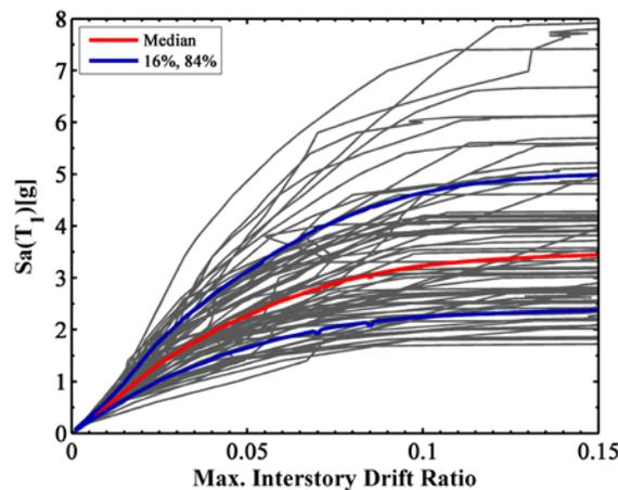
Fig. 2 – IDA curves of the 3-story structure with the supplemental viscous damping ratio of 0.1
