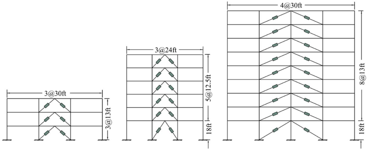
Fig. 1– Dimensions of the SMRFs and the configuration of linear FVDs in the SMRFs with linear FVDs
