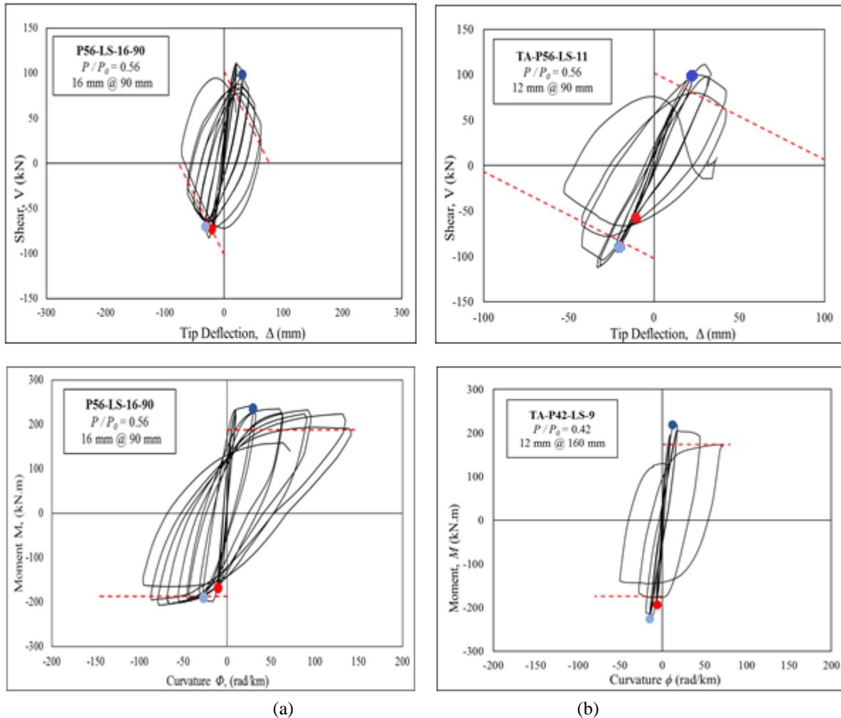
Fig. 7 - Shear vs. Deflection and Moment vs. Curvature relations of columns under higher axial load level: (a) Circular Column (Specimen No. 11); and (b) Square Column (Specimen No. 3)
