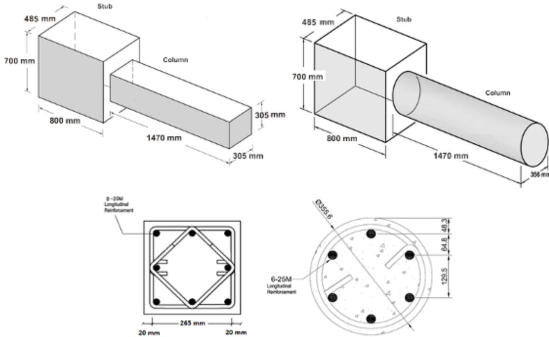
Fig. 2 - Schematics and cross-sections of square and circular specimens
