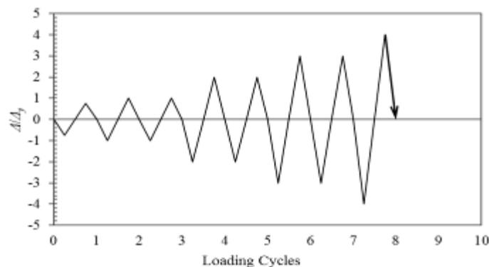
Fig. 4 - Typical Transverse Displacement History
