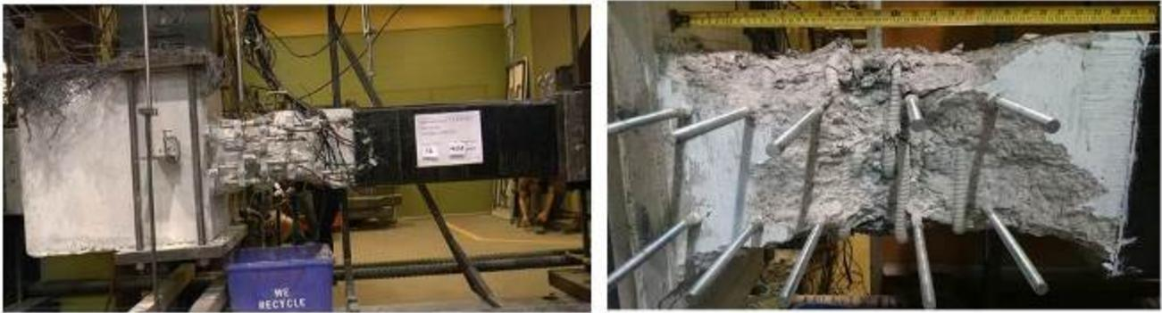
Figure 5. A typical column during testing and at failure
