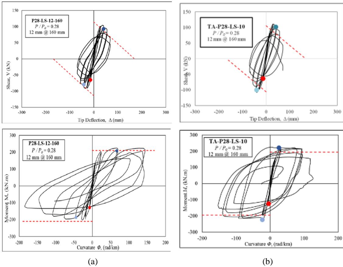
Fig. 6 - Shear vs. Deflection and Moment vs. Curvature relations for columns under lower axial load level
