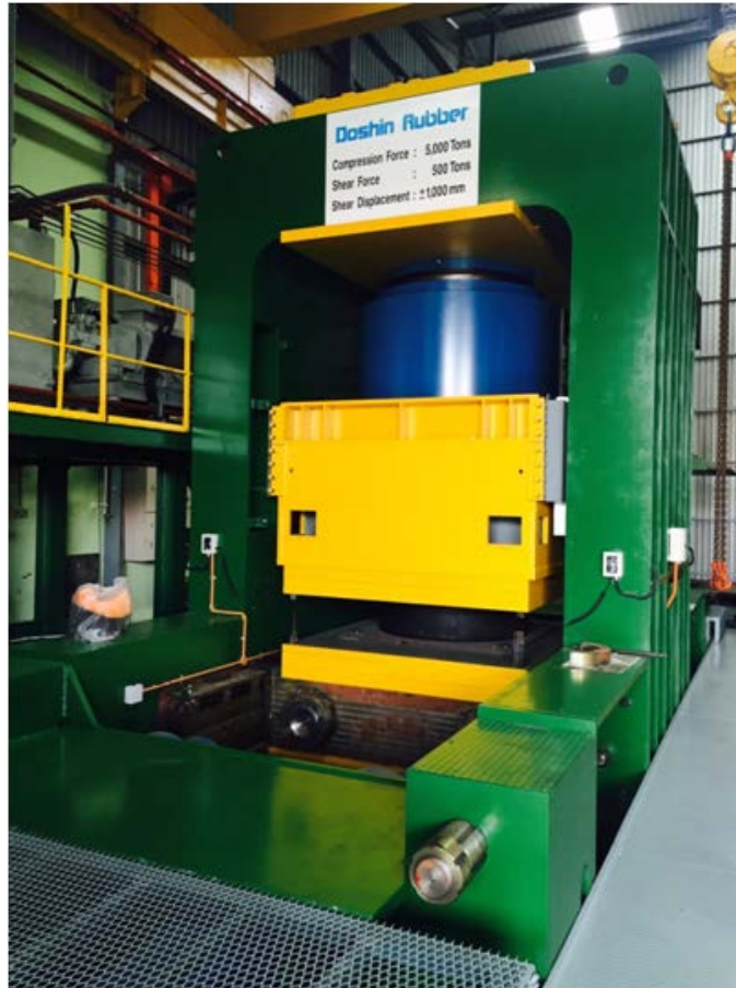
Fig.4 eLab-150 testing machine – one of the world’s largest
