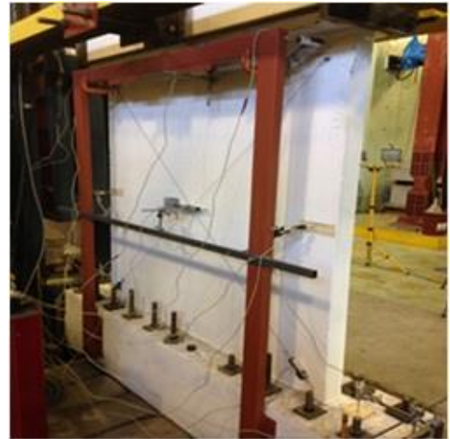
b) Steel frame for the instrumentation
