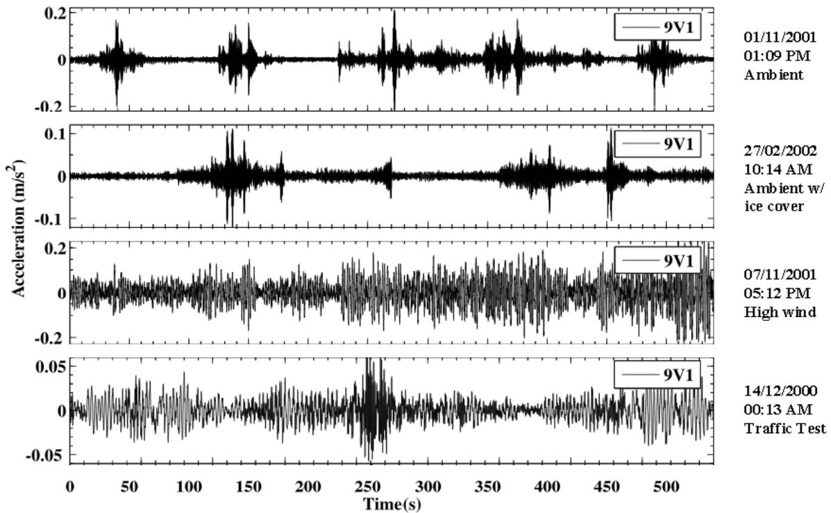
Fig. 2. – Typical vertical acceleration time histories under different loading scenarios
