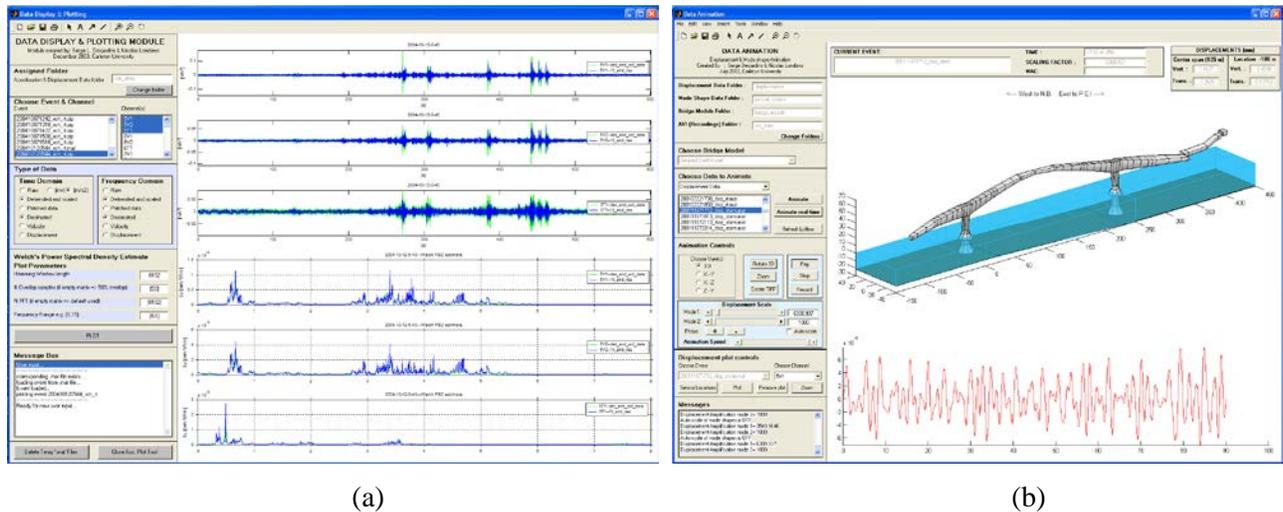
Fig. 3 – Graphical user interfaces (a) data display module; (b) animation module
