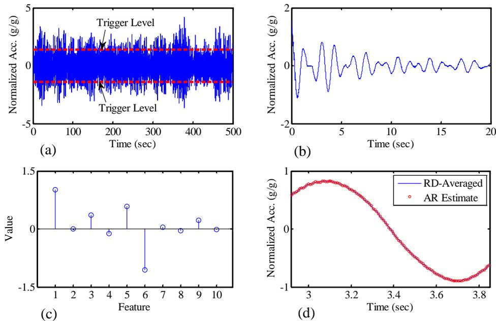
Fig. 7 – Autoregressive model applied to dataset DS1 with RD averaging: (a) standardized acceleration time-history; (b) RD-averaged signal; (c) extracted features; (d) comparison of AR estimate and RD-averaged signal.
