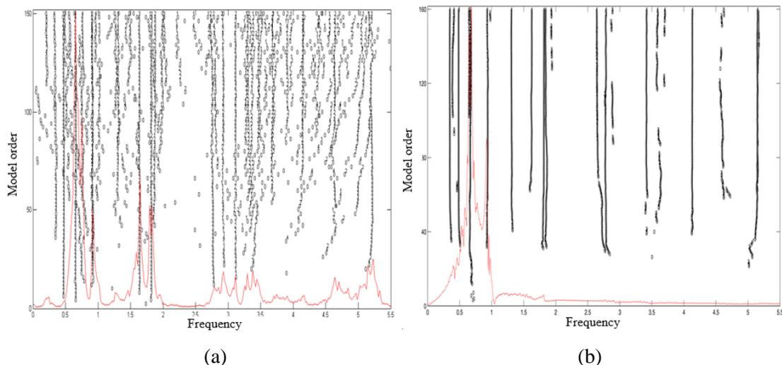
Fig. 4. – Stabilization diagram: (a) SSI method; (b) PolyMAX method
