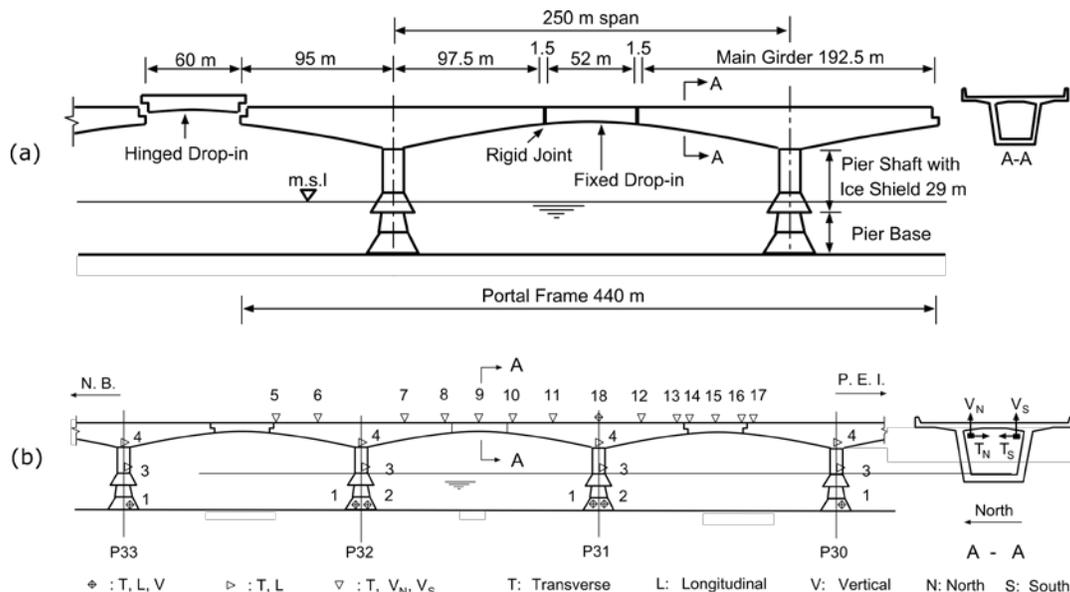
Fig. 1 – (a) Dimensions, main components; (b) Accelerometer locations in Confederation Bridge
