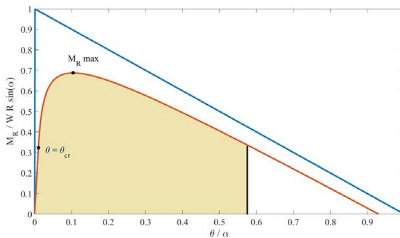
Fig. 3 – Calculation of the demand of the smooth block as the area underneath its moment-rotation curve
