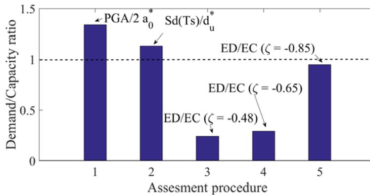
Fig. 8 - Demand/Capacity ratios for different approaches
