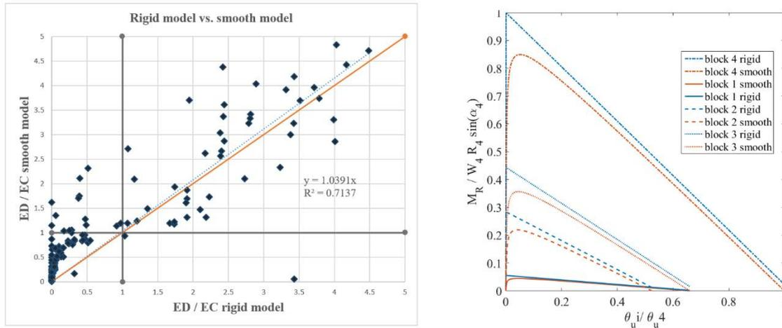
Fig. 4 - Comparison between the smooth and rigid model in terms of demand/capacity ratios (a) capacity curves for the four blocks considered (b)
