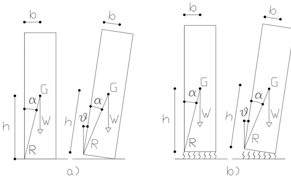
Fig. 1 – Comparison between the rigid model and the smooth model
