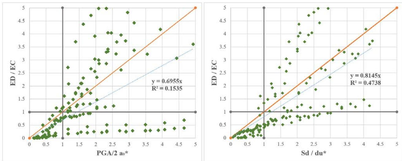
Fig. 5 - Comparison between the smooth model and code demand/capacity ratios (a) force-based and (b) displacement-based
