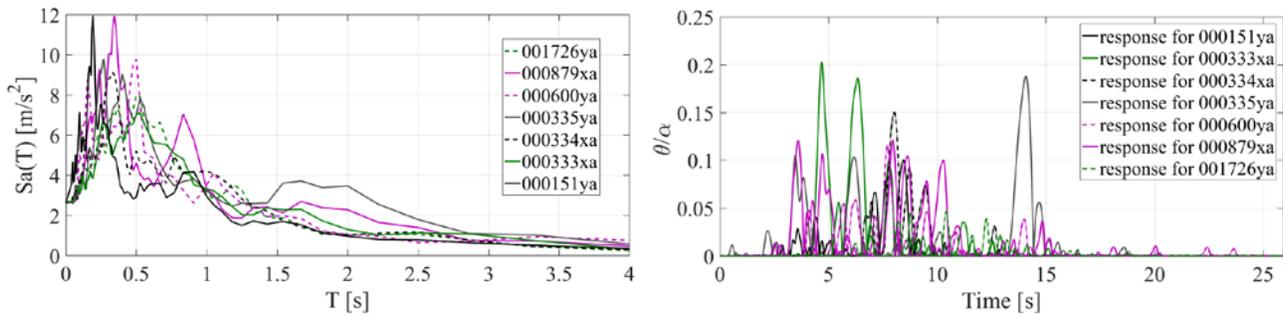
Fig. 7 - Time histories spectrums a) and one-sided rocking responses of the facade b)
