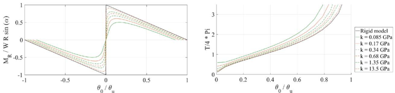
Fig. 2 – Moment rotation relationship a) and period b) for different values of  $k$
