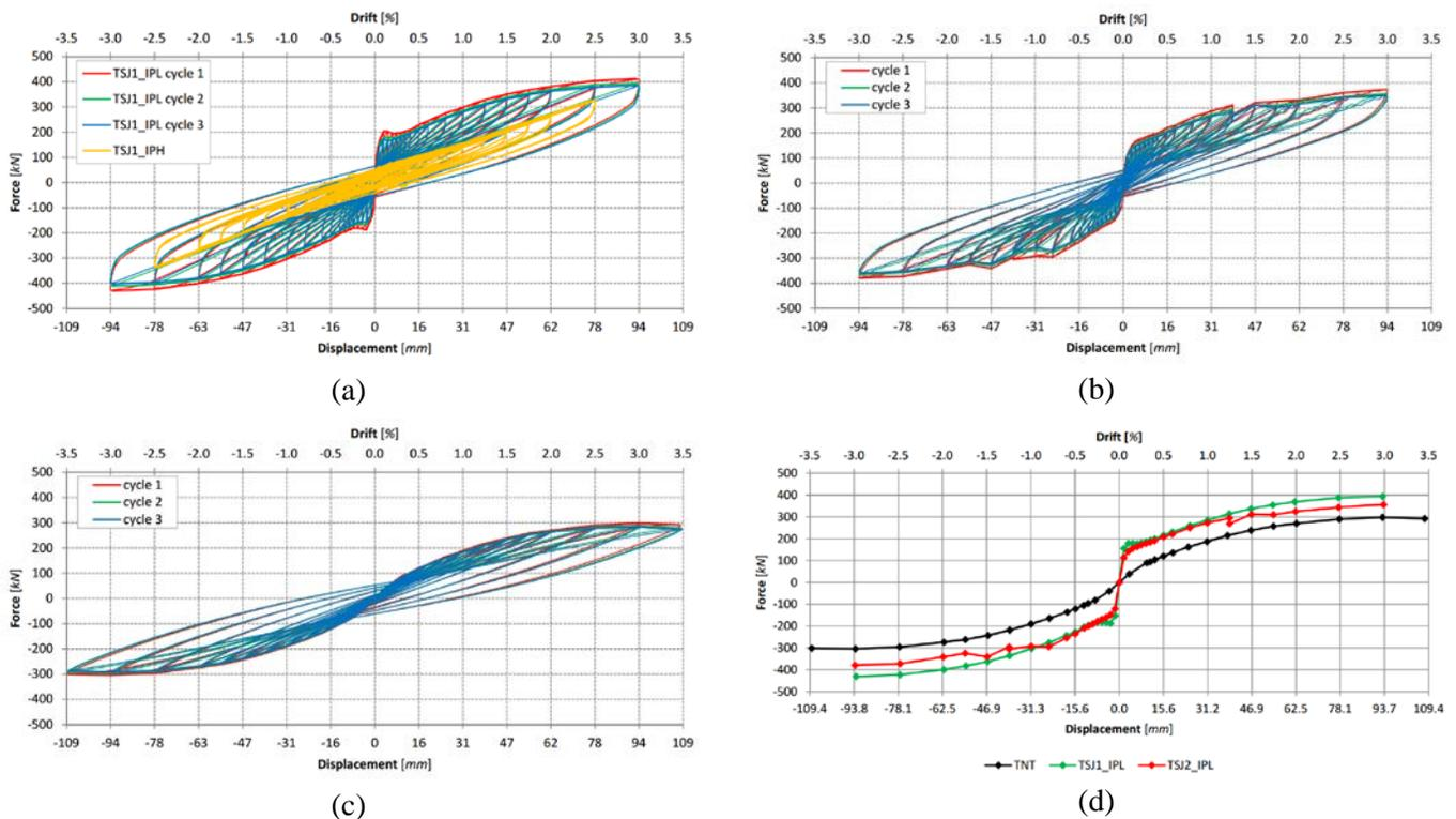
Fig. 4 – Force-displacement curves on (a) TSJ1 , (b) TSJ2, (c) TNT and (d) comparison of maximum envelopes.
