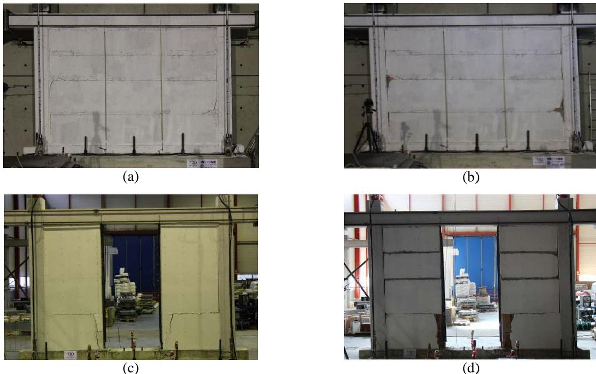
Fig. 5 – Damage pattern of TSJ1 at (a) 1.25% and at (b) 3.00% drift ; damage pattern of TSJ2 at (c) 1.25% and at (d) 3.00% drift.
