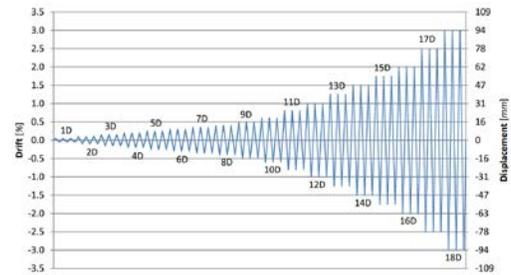
Fig. 3 – (a) Layout of the in-plane setup for cyclic tests; (b) in-plane testing protocol for TSJ1 and TSJ2 (“low” velocity test).
