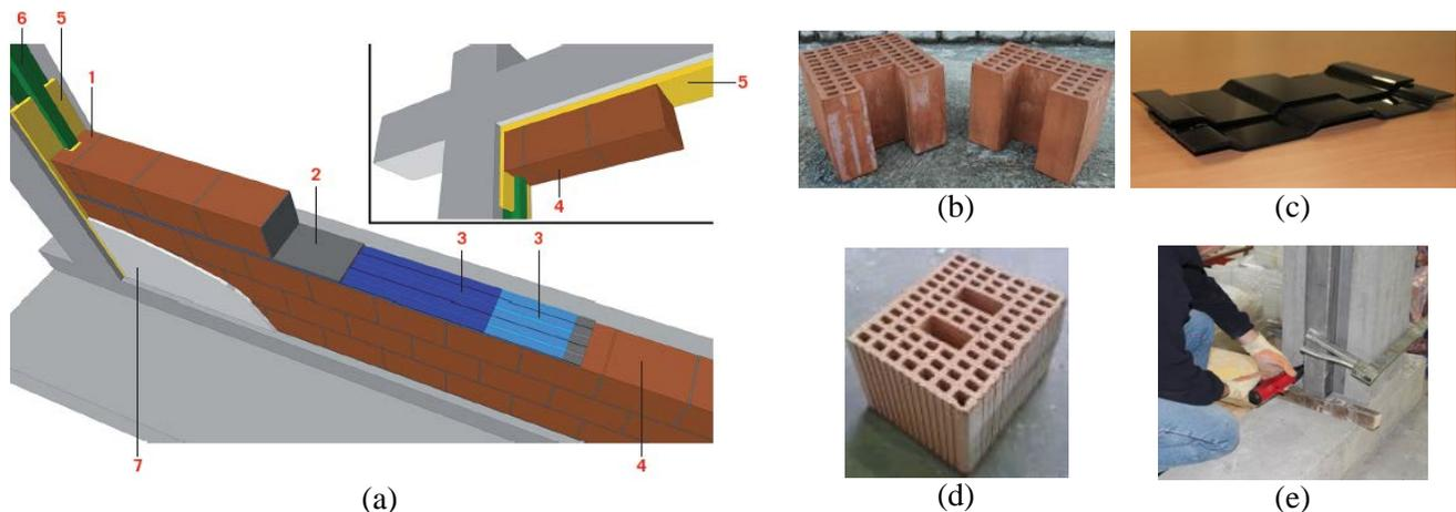
Fig. 1. – (a) Details of the innovative masonry infill with sliding joints: 1. (b) C-shape units; 2. mortar bed-joints; 3. (c) sliding joints; 4. (d) clay units; 5. interface joints; 6. (e) shear keys; 7. plaster.
