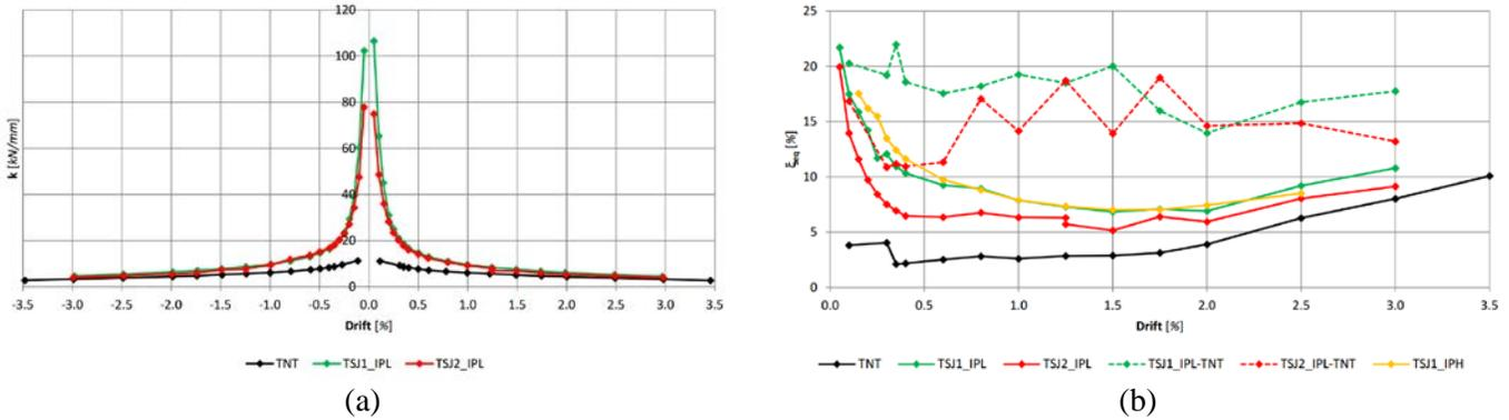
Fig. 7 – (a) Stiffness degradation vs imposed drift of TNT, TSJ1 and TSJ2 at 1<sup>st</sup> cycles; (b) equivalent viscous damping of TNT, TSJ1 (for “low” and “high” velocity tests), TSJ2, TSJ1-TNT and TSJ2-TNT at 1<sup>st</sup> cycles.
