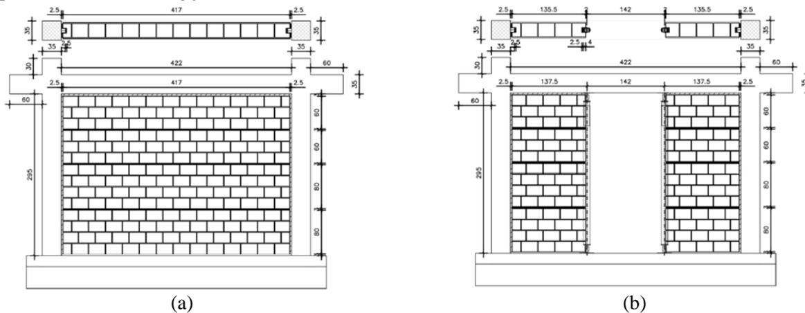
Fig. 2 – Layout of the (a) fully infilled (TSJ1) and of the (b) partially infilled (TSJ2) RC frame specimens (represented without plaster).
