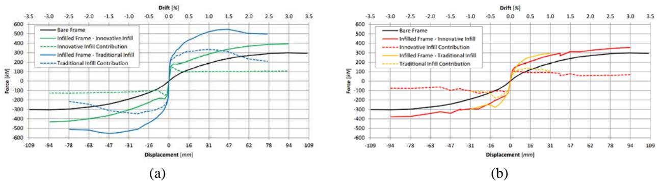
Fig. 8 – Force-displacement average envelope curves: (a) comparison between bare frame, innovative and traditional full infill; (b) comparison between bare frame, innovative infill and traditional infill with opening.
