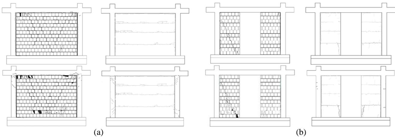
Fig. 9 – Comparison of the damage pattern between traditional and innovative infill: (a) fully infilled frame at 0.50% and 1.75% drift; (b) infill with opening at 0.35% and 1.00% drift.
