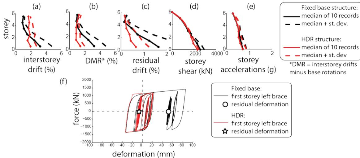
Figure 6: Results of nonlinear timehistory analysis for DBE suite: (a) interstorey drift; (b) interstorey drift minus base rotation (DMR); (c) residual drift; (d) storey shear; (e) storey accelerations; (f) first storey left brace hysteresis
