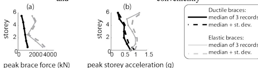
Figure 1: Response of ductile and elastic rocking frames to three records scaled to DBE (a) peak brace forces; (b) peak storey accelerations (analysis details are provided in Section 4.2)
