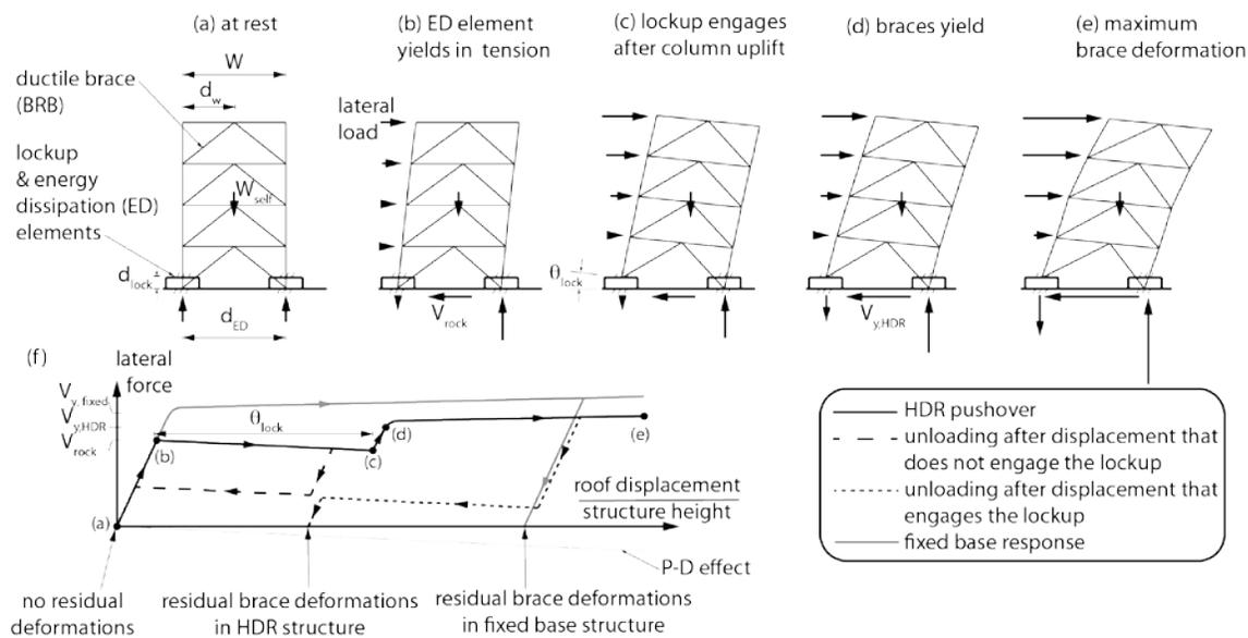
Figure 2: Overview of HDR mechanics: (a) schematic frame at rest; (b) energy dissipation element yields; (c) lockup engages after column uplift; (d) braces yield; (e) maximum brace deformation; (f) schematic force-deformation plot for HDR system
