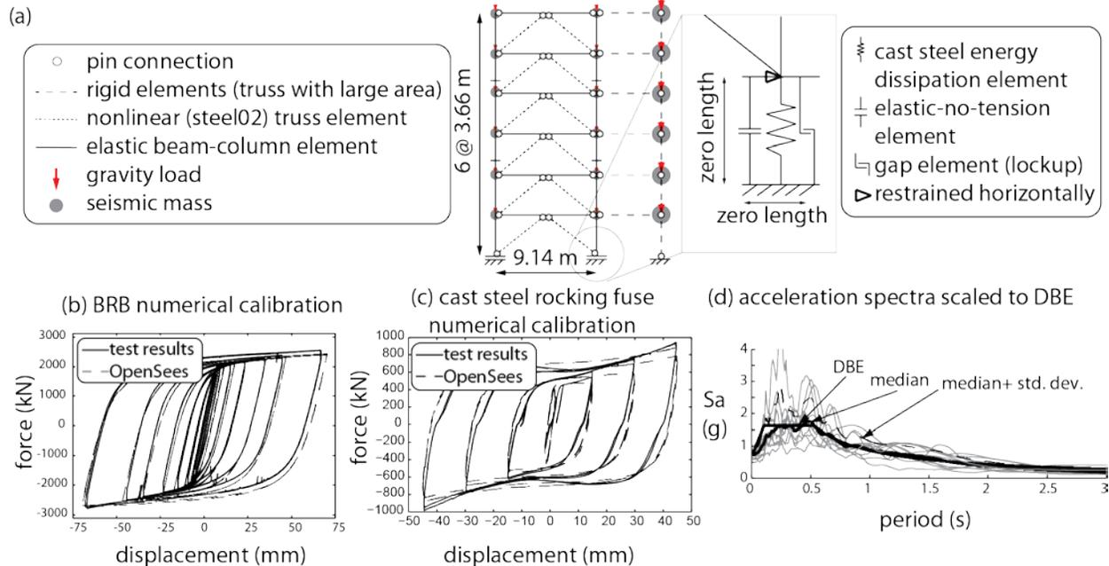
Figure 5: Numerical modelling and analysis: (a) modelling assumptions; (b) calibration of buckling-restrained brace elements to tests [17]; (c) calibration of cast steel supplemental energy dissipation elements to tests performed at the University of Toronto in 2014
