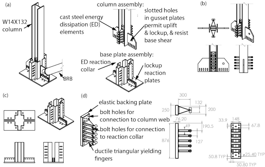
Figure 4: HDR column-foundation detail: (a) overview; (b) column assembly; (c) base plate assembly; (d) cast steel energy dissipation element
