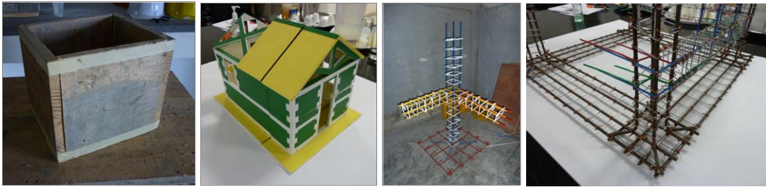
Fig. 4: 3D demo objects for classroom training: a) Role of ring beam, b) how to read cross sections, c) full scale model of reinforcement (oprepared by BuildChange), d) 1:10 scale model of reinforcement)
