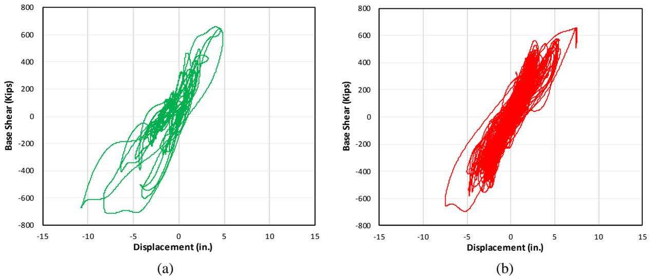
Fig. 11 – Six Story CBF force-displacement (hysteresis) due to both (a) crustal and (b) subduction records
