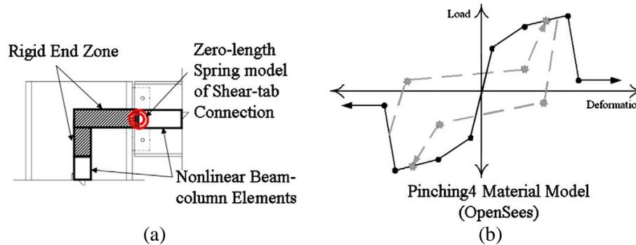
Fig. 3 - Illustration of (a) the shear-tab connection, after [1], and (b) the Pinching4 material model in OpenSees.
