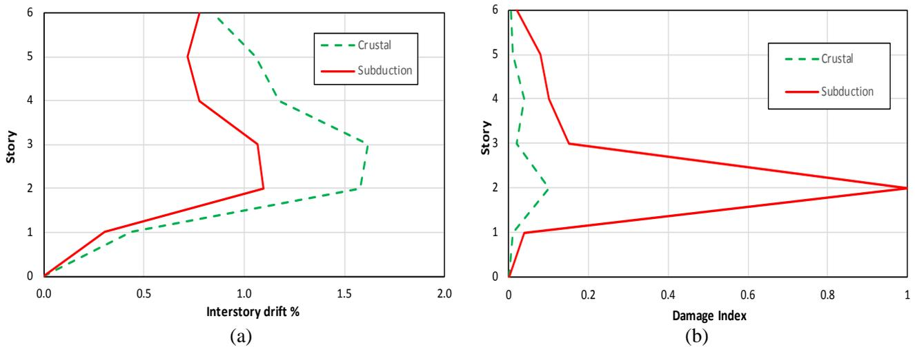
Fig. 10 – (a) Interstory drift profile and (b) Damage Index of the outermost compression fiber of HSS braces, under both subduction and crustal records
