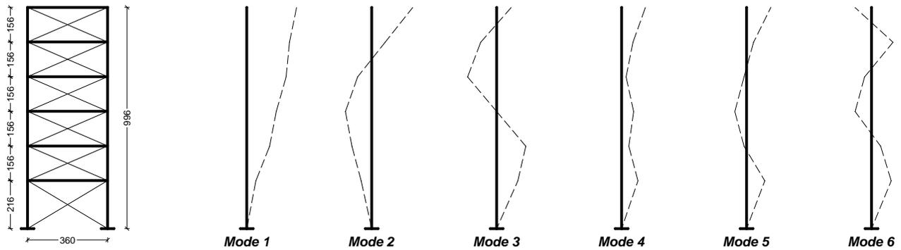
Fig. 9 - Six story (X-braced) CBF under study and the first six mode shapes.
