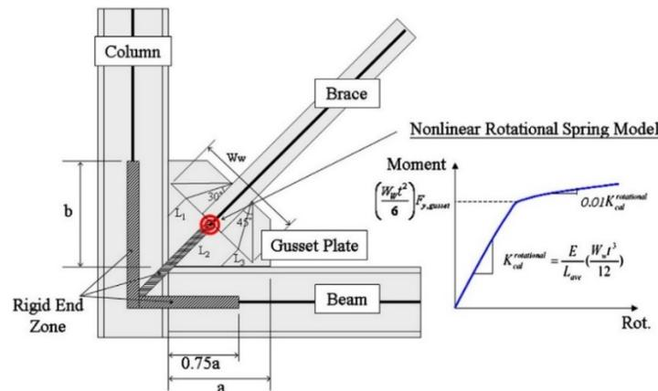
Fig. 2 – Illustration of the proposed connection model after Hsiao et al. [1].
