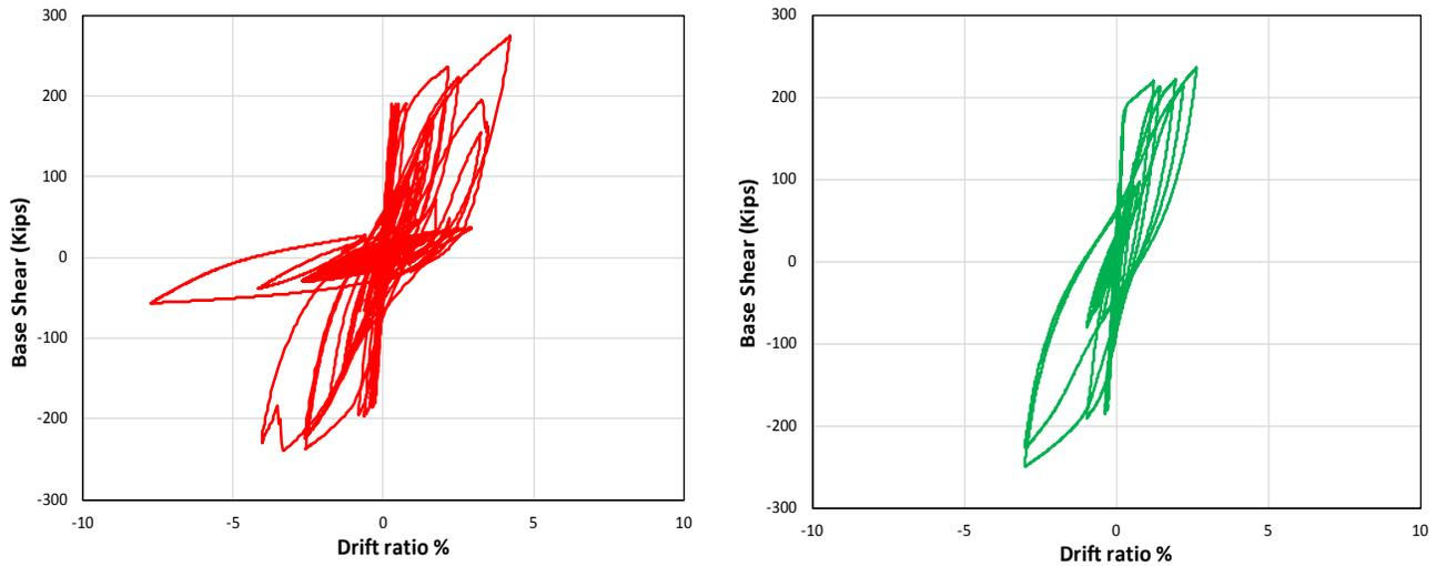
Fig. 7 – Single Story CBF force-deformation relationship (hysteresis) due to the 100% scale of short (right) and long (left) ground motions.
