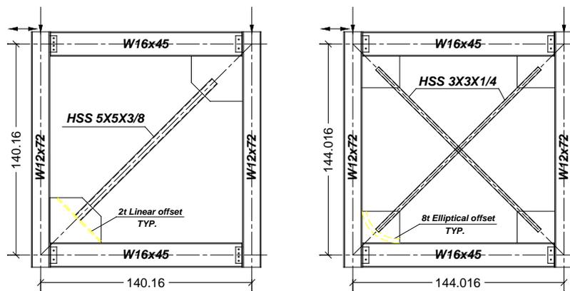
Fig. 1 - Typical test specimen for single-story single-bay SCBF: diagonal-braced HSS1 (left) and X-braced HSS31 (right).
