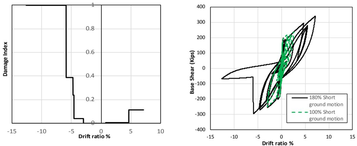
Fig. 8 – Single story CBF response to 180% scale of short duration ground motion.
