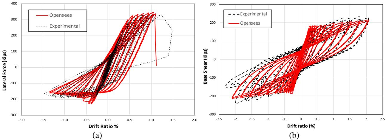
Fig. 4 - Simulated and measured responses of specimens (a) HSS1 and (b) HSS31.
