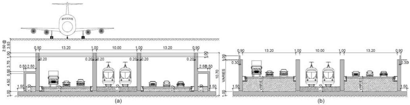
Fig. 4 – (a) Typical Cross Section of Tunnel. (b) Typical Cross Section of Ramp (unit: m).
