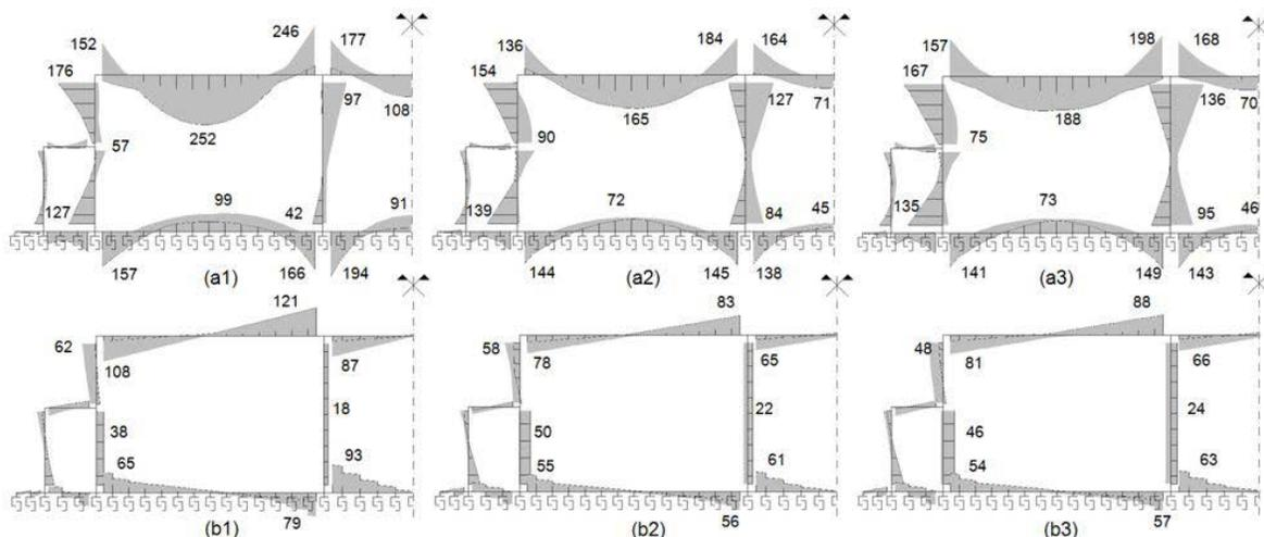
Fig. 8 – (a) Bending moment envelopes (unit: t-m/m); (b) Shear force envelopes (unit: t/m). (1) Strength I; (2) Extreme Event I (M-O); (3) Extreme Event I (Raking).
