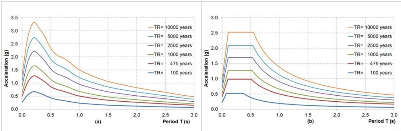
Fig. 3– (a) Uniform hazard spectrums. (b) Design spectrums.
