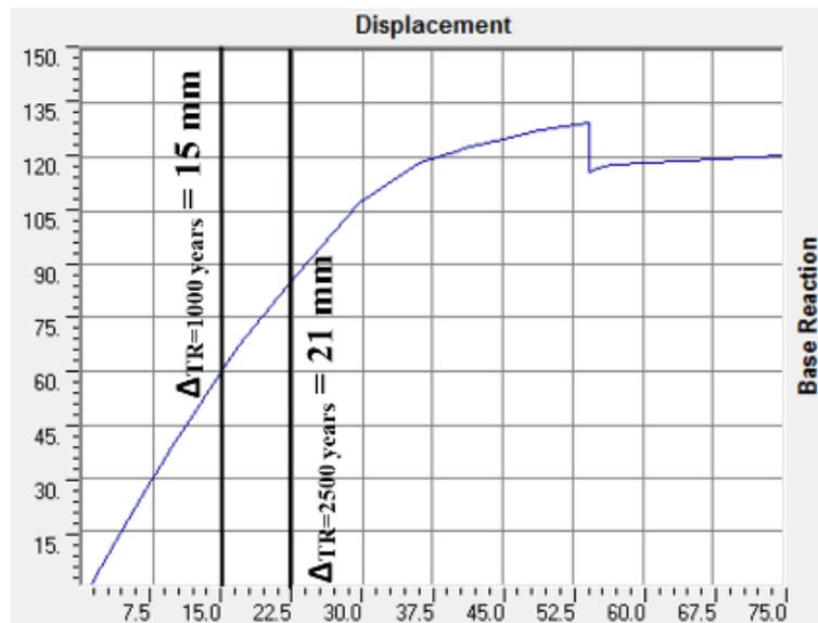
Fig. 11 – Pushover curve of typical tunnel section.
