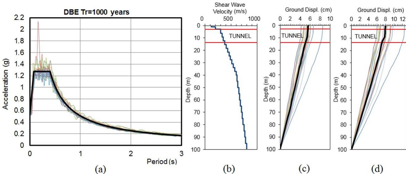
Fig. 7 – (a) Target spectrum and spectrum of 20 spectrum-matched ground motions for 1000-year return period hazard level in site class B. (b) Shear wave velocity profile. (c) Mean relative displacement of the ground for 1000-year return period earthquake. (d) Mean relative displacement of the ground for 2500-year return period earthquake.
