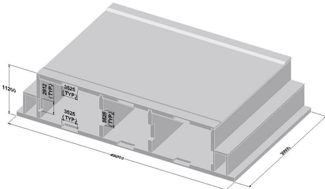
Fig. 10 – Shear Key concept for the tunnel section. Units in millimeters.
