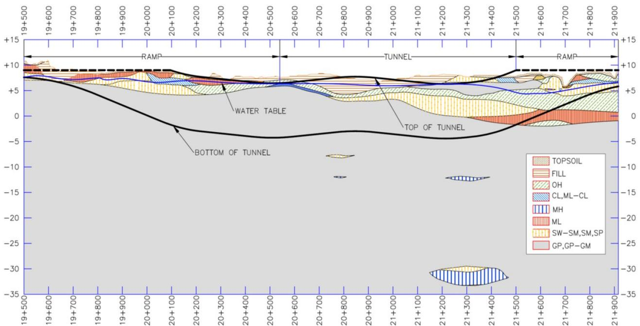
Fig. 2 – Geological profile and project alignment.
