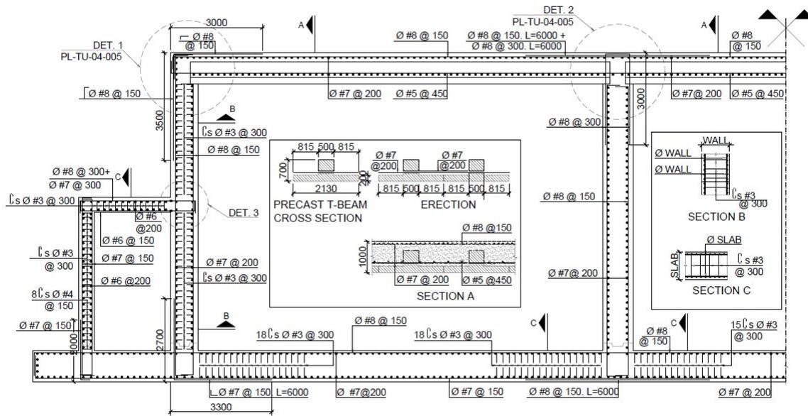
Fig. 9 – Typical Reinforcement Details of the tunnel section. Precast T-Beam reinforcement not shown for clarity.
