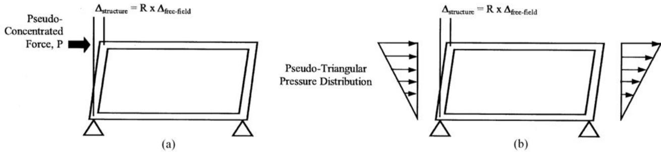
Fig. 6 – Simplified Frame Analysis Model (Wang [4]): (a) pseudo-concentrated force at the corner; (b) pseudo-triangular pressure distribution on the side walls.
