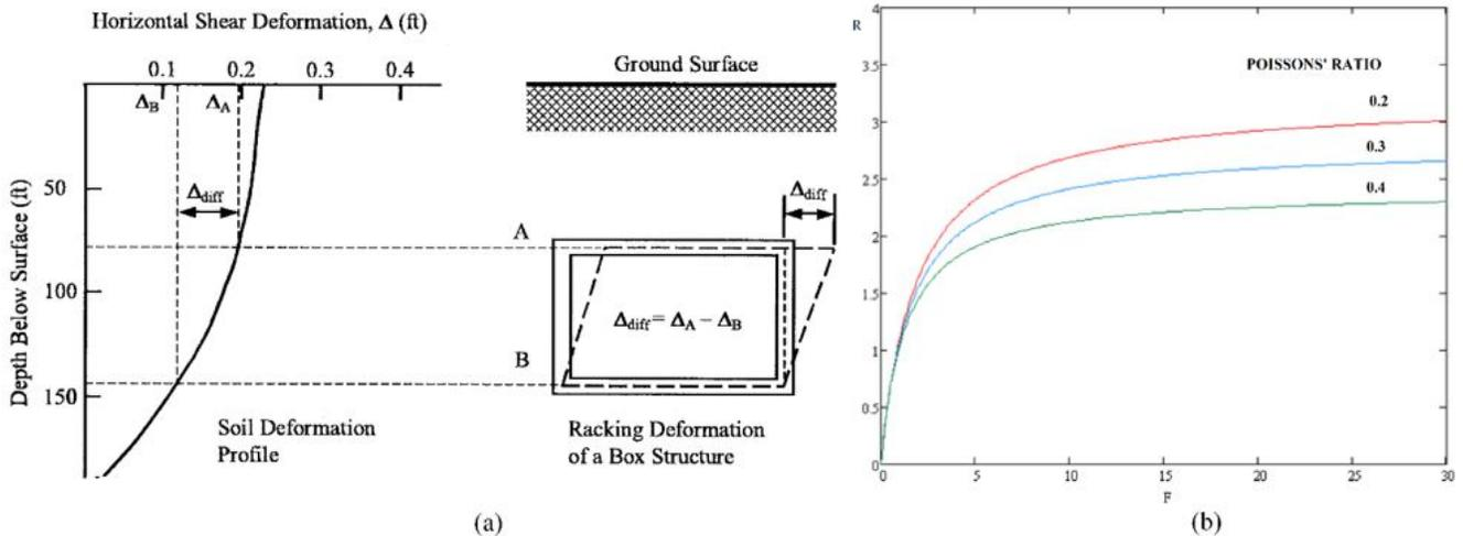
Fig. 5 – (a) Racking Deformation of a Box Structure; (b) racking coefficient. (Wang 1993 [4]).
